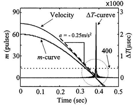
Fig. 3. Number of encoder pulses  $m$  and auxiliary period  $\Delta T$  at low velocity (simulation).
