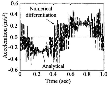
Fig. 5. Analytic and numerical differentiation based accelerations for sine-wave velocity profile with amplitude of 0.04 m/s and frequency of 1 Hz.
