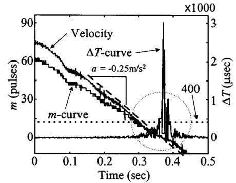
Fig. 4. Number of encoder pulses  $m$  and auxiliary period  $\Delta T$  at low velocity (experiment).
