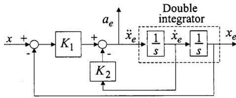
Fig. 8. Block diagram of low-acceleration estimator.
