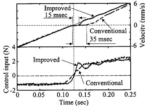
Fig. 15. Velocity responses and control signals for conventional PI controller (dashed) with proportional gain  $K_P = 60$ , integral gain,  $K_I = 2000$ , and friction compensation controller with LAE (solid) with acceleration gain  $K_a = 25$  ( $Vs^2/m$ ), where V is volt.
