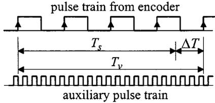
Fig. 2. Timing diagram of velocity measurement using M/T method.
