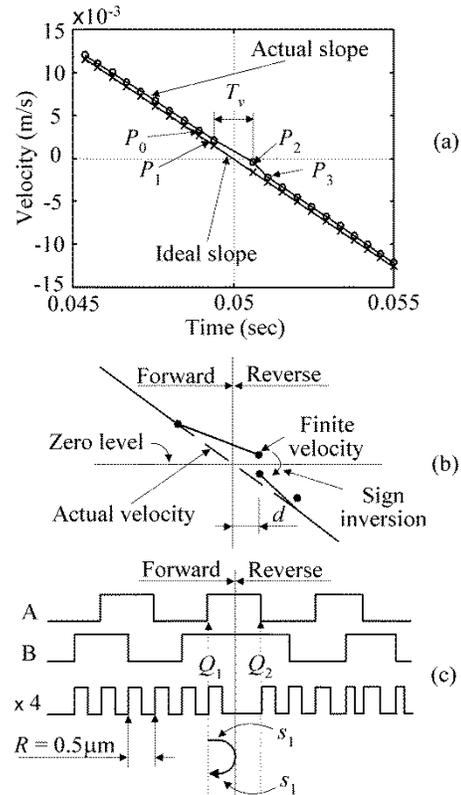
Fig. 7. Velocity detection around zero velocity by M/T method.
