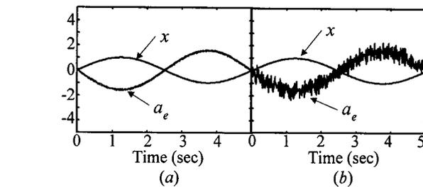
Fig. 12. Estimated acceleration responses for different bandwidths: (a)  $\omega_b = 50$  Hz,  $\zeta = 0.707$  and (b)  $\omega_b = 150$  Hz,  $\zeta = 0.707$ .
