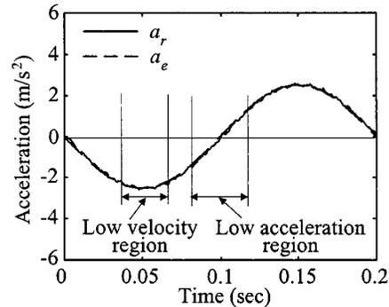
Fig. 10. Analytic and LAE-based accelerations for sinewave velocity profile with amplitude of 0.04 m/s and frequency of 5 Hz.
