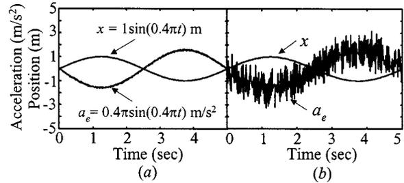
Fig. 9. Estimated acceleration responses of the PD controller: (a) excluding  $dx/dt$  in the derivative term and (b) including  $dx/dt$  in the derivative term.
