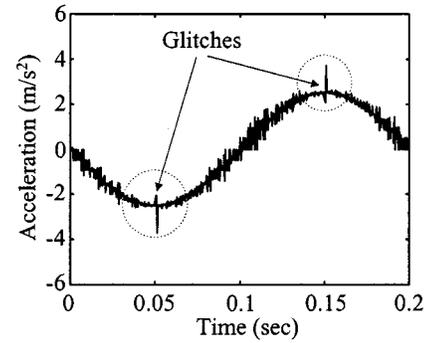
Fig. 6. Analytic and numerical differentiation based accelerations for sine-wave velocity profile with amplitude of 0.04 m/s and frequency of 5 Hz.
