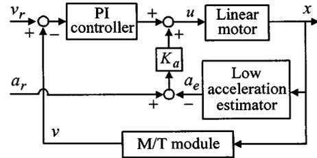
Fig. 14. PI velocity control system with LAE.
