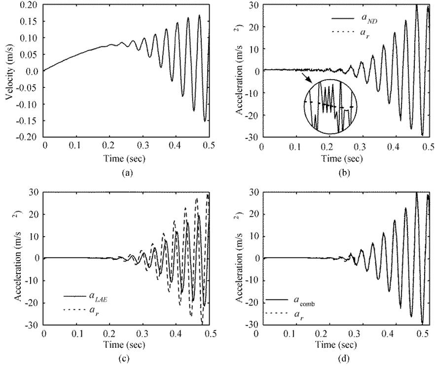
Fig. 13. Estimated accelerations of various estimation methods: (a) velocity profile, (b) acceleration by ND, (c) acceleration by LAE with  $\omega_b = 50$  Hz,  $\zeta = 0.707$ , and (d) acceleration by a combination of ND and LAE ( $V_{\min} = 0.0012$  m/s,  $C = 0.05$ ).
