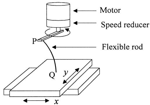
Fig. 15. Test apparatus for active mass implementation.
