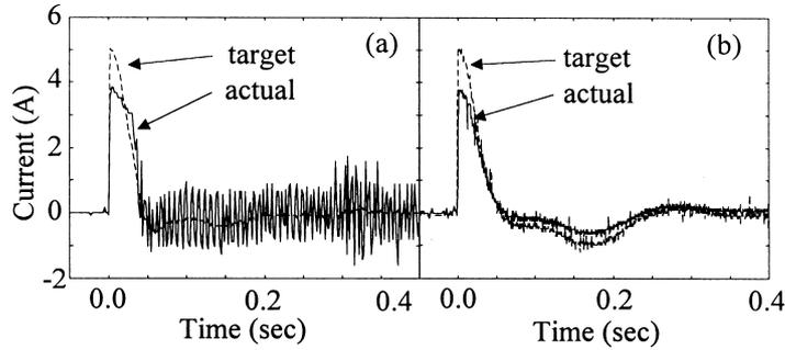
Fig. 5. Current responses with PID controller; (a) high P gain and (b) low P gain.
