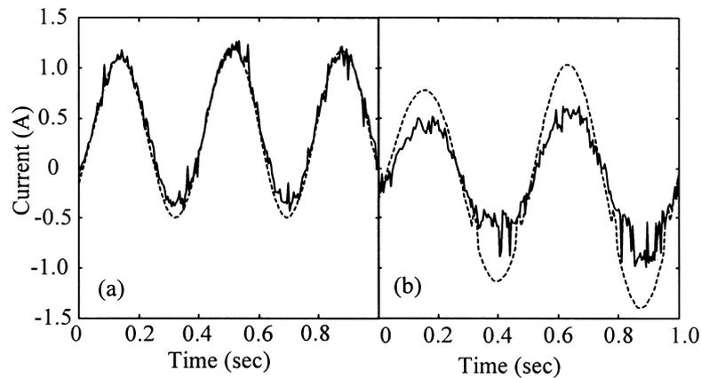
Fig. 12. Current responses of arm motion generator with active stiffness implemented: (a) 2-DOF controller, and (b) PI controller.
