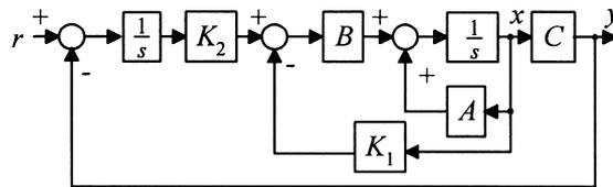
Fig. 10. Block diagram of LQ-servo controller.
