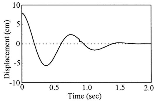
Fig. 13. Displacement response of the motion generator subject to initial displacement with active stiffness implemented.
