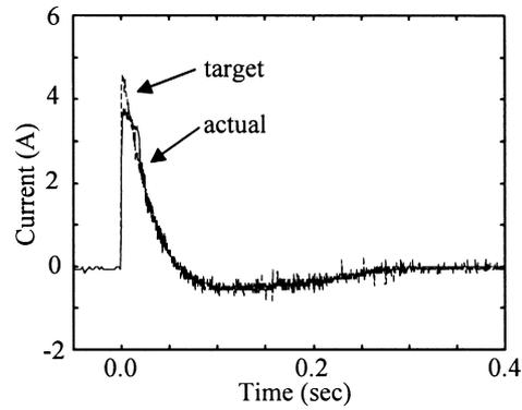
Fig. 11. Current response with 2-DOF controller.
