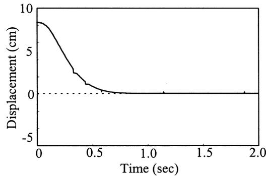
Fig. 14. Displacement response of the motion generator subject to initial displacement with active stiffness and damping implemented.
