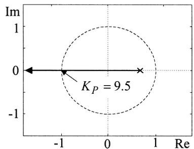
Fig. 4. Root locus of discretized electric part.
