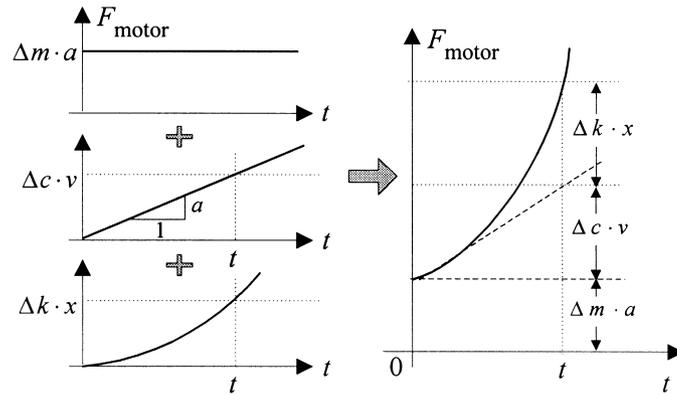
Fig. 3. Motor forces required for active inertia, damping and stiffness during uniformly accelerated motion.
