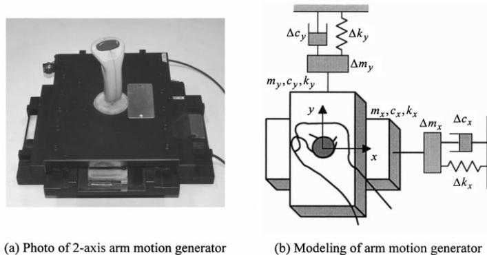
Fig. 1. Configuration of motion generator and concept of active impedance.
