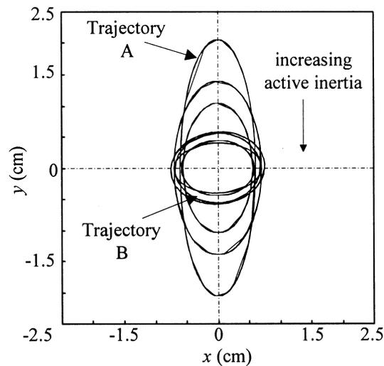
Fig. 16. Change in trajectory of the lever as the amount of active mass increases (trajectory A is without active mass implemented).
