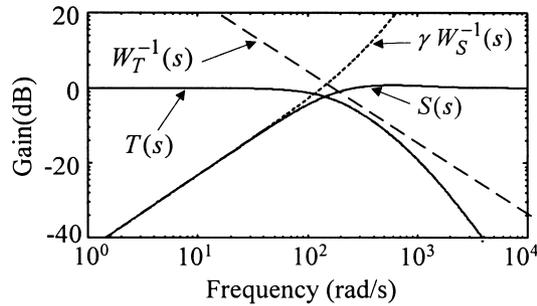
Fig. 9. Sensitivity, cosensitivity functions and their inverse weighing functions.
