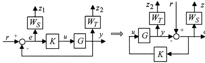
Fig. 8. Mixed sensitivity H-infinity problem with weighing functions.
