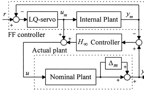
Fig. 6. Block diagram of 2-DOF current controller composed of LQ-servo and H-infinity controllers.
