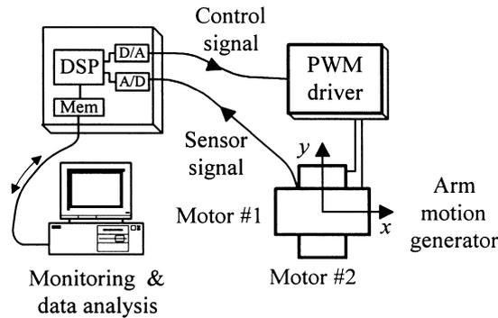
Fig. 2. Schematic experimental setup.
