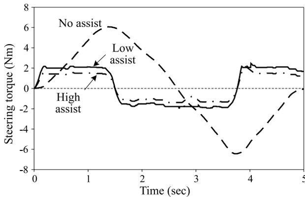
Fig. 11. Steering torque with sinusoidal steering input.
