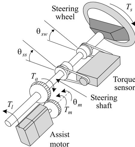
Fig. 4. Configuration and free-body diagram of a steering column.
