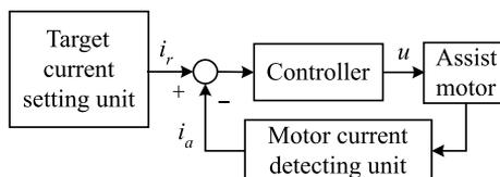
Fig. 1. Block diagram of typical EPS control system.
