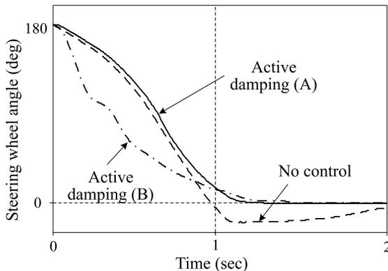
Fig. 13. Responses of steering wheel angle with active damping control activated.
