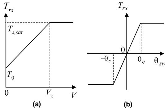
Fig. 8. Determination of reference steering torque depending on (a) vehicle speed and (b) steering wheel angle.
