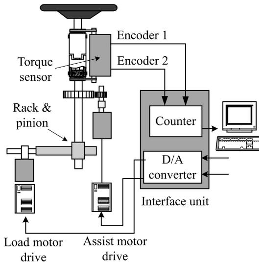
Fig. 2. Experimental setup used to implement EPS control logic.
