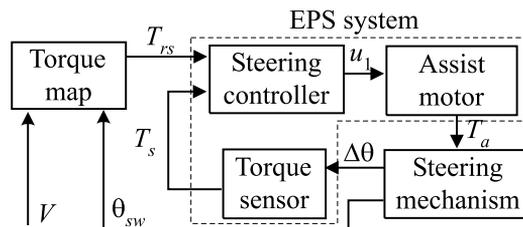
Fig. 7. Block diagram of control logic for reduction in steering torque.
