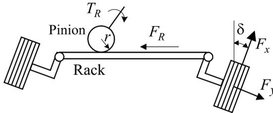
Fig. 5. Simplified model of steering rack and pinion system.
