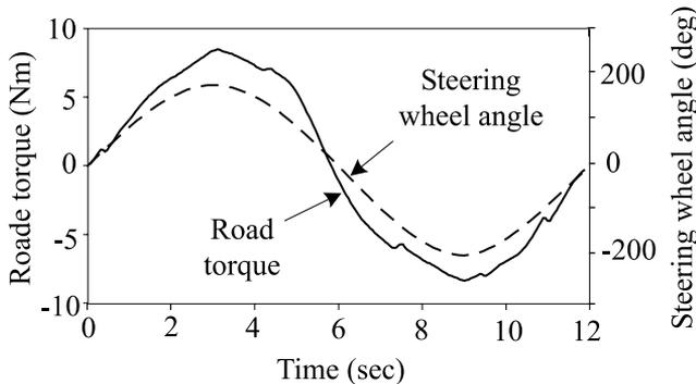
Fig. 6. Road torque versus steering wheel angle (experimental data).
