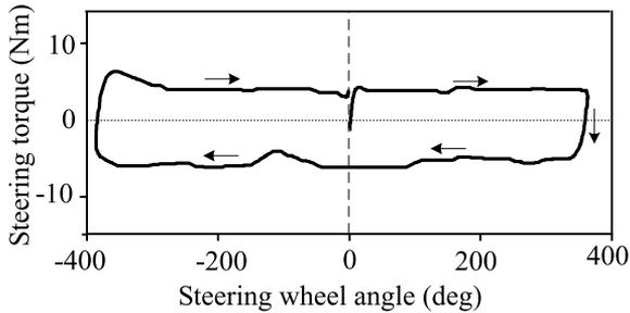
Fig. 12. Plot of steering torque versus steering wheel angle.
