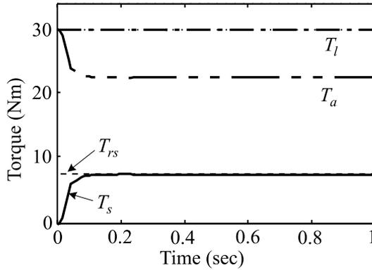
Fig. 10. Time responses of steering torque and assist torque for constant load torque and vehicle speed.
