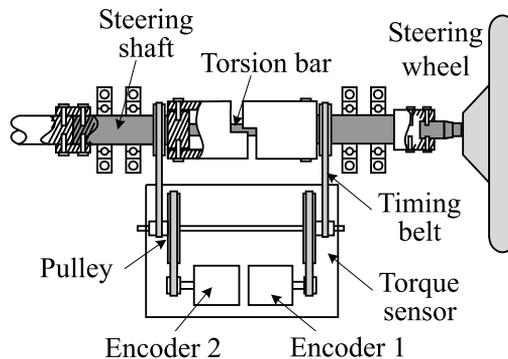
Fig. 3. Structure of a torque sensor.
