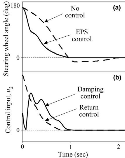
Fig. 14. Responses of steering wheel angle and control inputs with both damping and return control controls activated.
