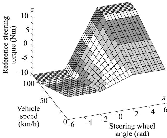
Fig. 9. Three-dimensional plot of proposed torque map.
