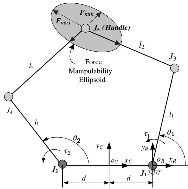
Fig. 1. Linkage mechanism for 2 DOF haptic device.
