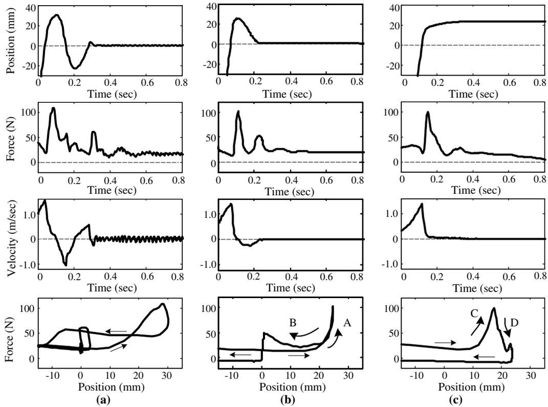
Fig. 9. Experimental results for contact with hard wall at high velocities: (a) active haptic system, (b) PO/PC based haptic system, and (c) hybrid haptic system.
