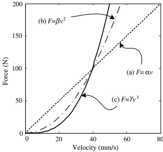
Fig. 7. Different dampers used in experiments: (a) linear damper, (b) and (c) nonlinear dampers.
