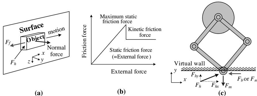
Fig. 10. Representation of friction effect: (a) friction model, (b) relationship between external force and friction force, and (c) forces acting on the system to represent friction.
