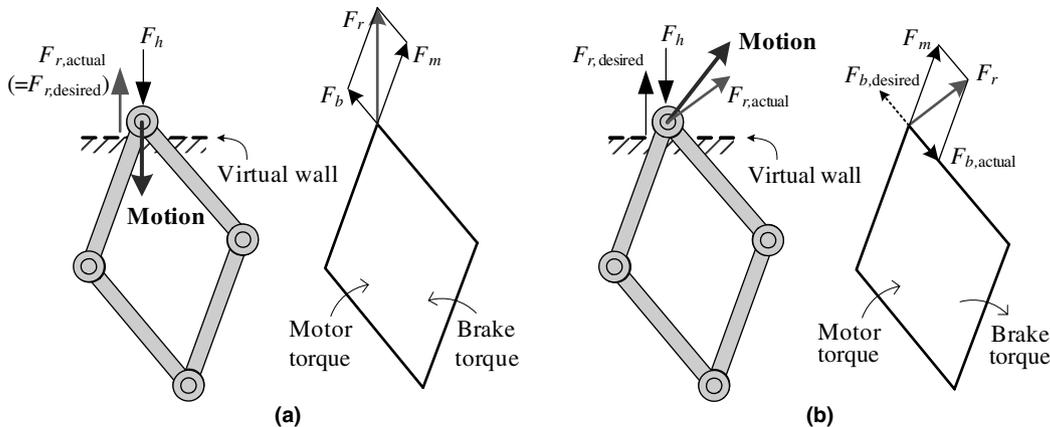
Fig. 5. Control of hybrid system: (a) compression of virtual wall and (b) release of virtual wall.
