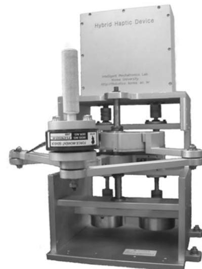
Fig. 3. Photo of hybrid haptic device.
