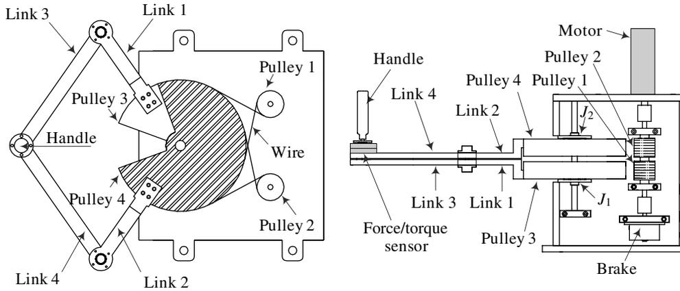
Fig. 4. Basic structure of hybrid haptic device.
