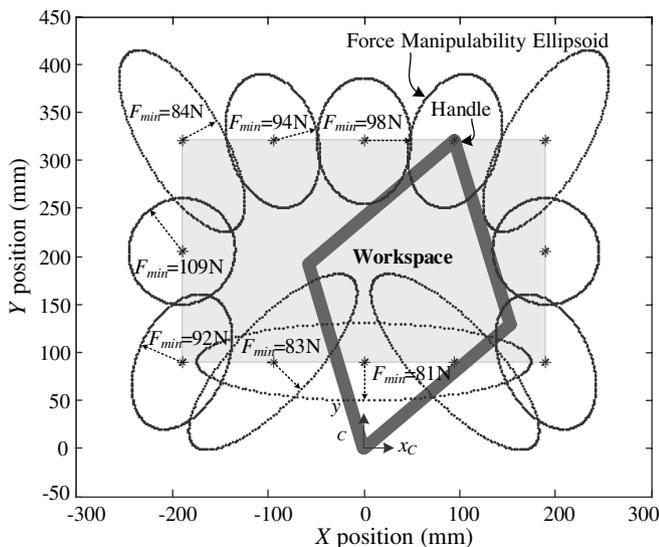
Fig. 2. FME simulation results for motor-driven device in whole workspace.
