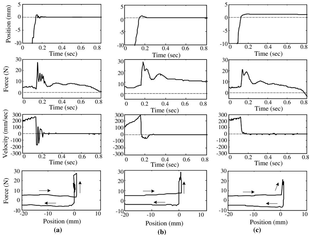
Fig. 8. Experimental results for contact with hard wall at low velocities: (a) active haptic system, (b) PO/PC based haptic system, and (c) hybrid haptic system.
