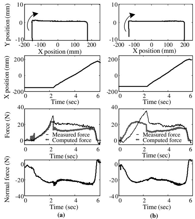
Fig. 11. Results for friction experiment with small normal force: (a) active haptic system and (b) hybrid haptic system.
