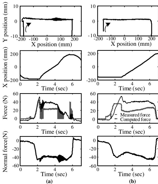
Fig. 12. Results for friction experiment with large normal force: (a) active haptic system and (b) hybrid haptic system.
