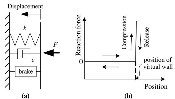
Fig. 6. Virtual wall model and ideal relation of force versus position during contact with stiff wall.
