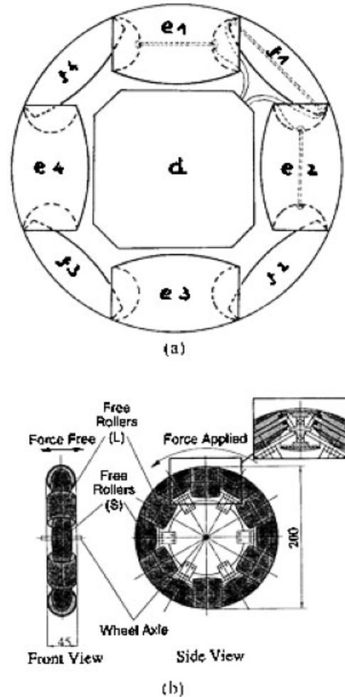
**Figure 2.** Various alternate wheels; (a) Fuchs and (b) Asama.
