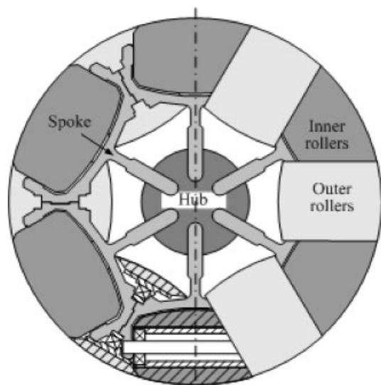
Figure 11. Schematic diagram of proposed continuous alternate wheel.
