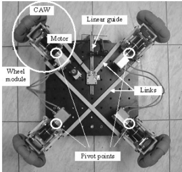
Figure 14. Bottom view of prototype vehicle with CAWs.
