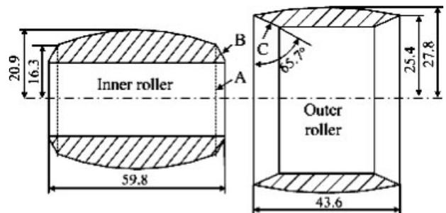
Figure 9. Final shapes of inner and outer rollers.
