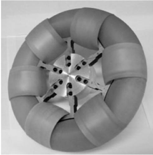
**Figure 12.** Photo of constructed continuous alternate wheel.
