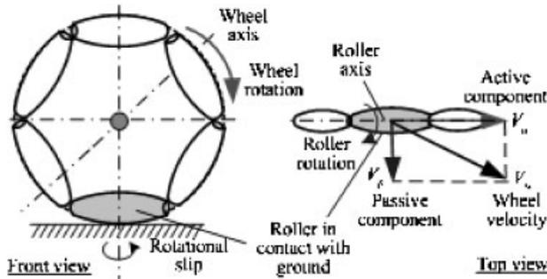
Figure 3. Three DOFs in a general omnidirectional wheel.
