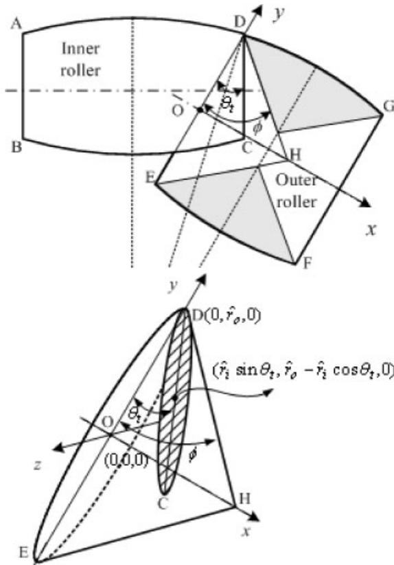
Figure 7. Interpenetration of inner roller into outer roller.
