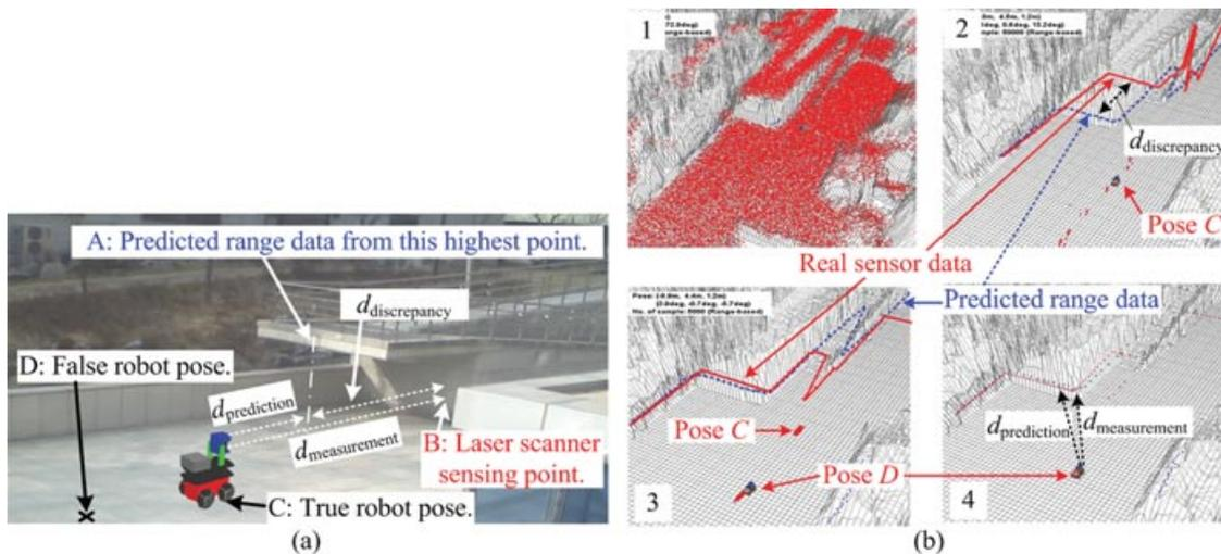
**Figure 4.** Incorrect convergence of samples during global localization because of discrepancy between elevation map and real range sensor data: (a) experimental environment and (b) convergence of samples.
