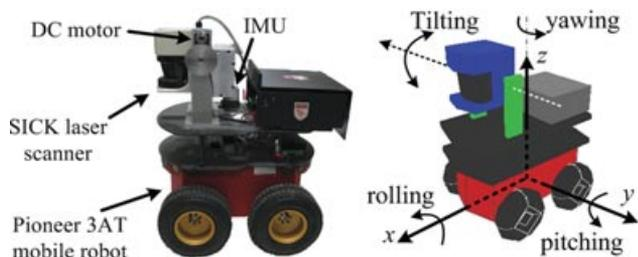
**Figure 5.** Robot used in the experiments.
