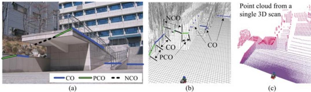
**Figure 9.** Experimental results of COAG feature extraction: (a) environment, (b) extraction result superimposed on elevation map, and (c) 3D point cloud.
