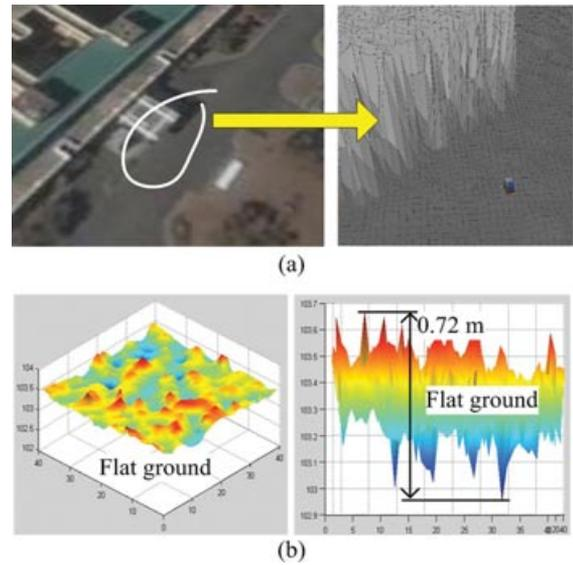
Figure 17. Examples of uncertainty of elevation map built by aerial mapping system: (a) roof and wall and (b) flat ground.
