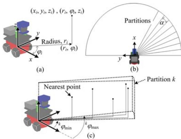
Figure 7. (a) Coordinate systems, (b) partitions divided at regular intervals, and (c) example of one partition including several sensing points.
