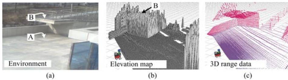
Figure 2. Examples of discrepancy between elevation map and real range sensor data.
