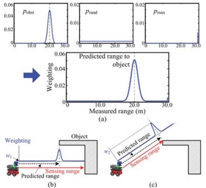
Figure 12. Weighting computation by sensor model: (a) sensor model, (b) unsuitable weighting computation for matching with unclassified sensing points, and (c) suitable weighting computation for matching with classified sensing point.
