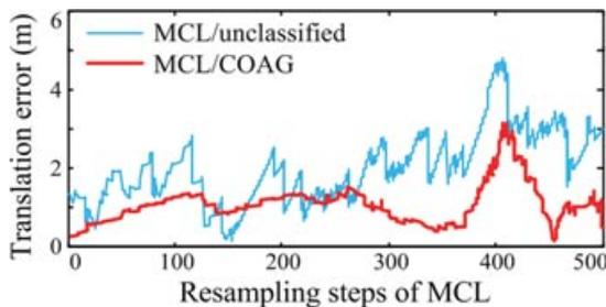
Figure 16. Translation errors between estimated positions and true positions.
