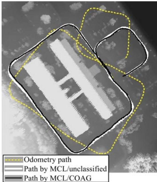
Figure 15. Paths estimated by odometry and MCL/COAG.
