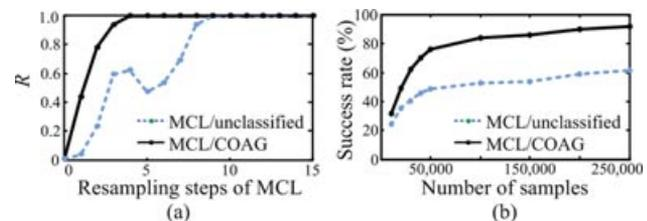
Figure 14. Characteristics of sample convergence: (a) sample convergence to correct pose versus resampling steps (initial number of samples: 100,000) and (b) success rate of global localization versus number of samples.
