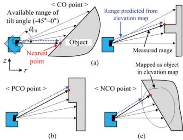
Figure 8. Classification of nearest point using sensing points included in one partition: (a) CO, (b) PCO, and (c) NCO.
