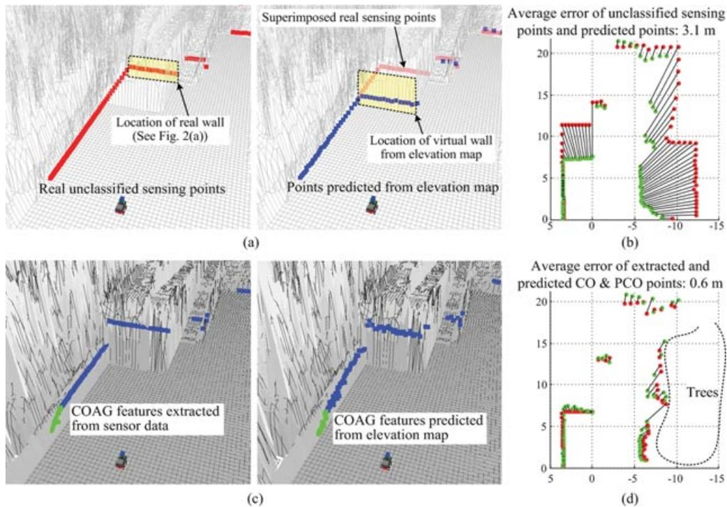
**Figure 10.** Comparison of real sensor data and predicted data: (a) unclassified range data and predicted range data, (b) average error of unclassified sensing points, (c) extracted COAG feature and COAG feature predicted from elevation map, and (d) average error of COAG features.
