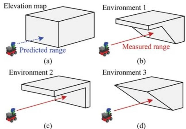
Figure 3. Examples of environments to be modeled as an identical elevation map.
