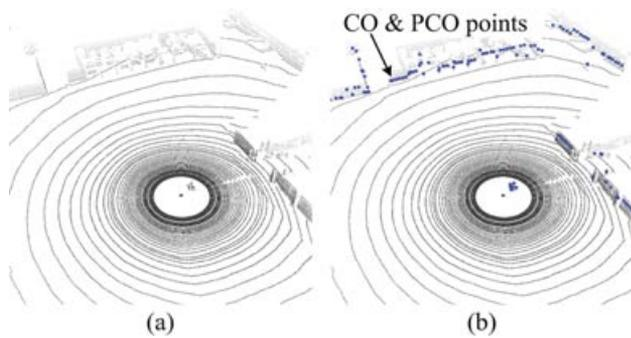
**Figure 18.** Feature extraction from 3D range data: (a) 3D range data from a Velodyne and (b) COAG feature points.
