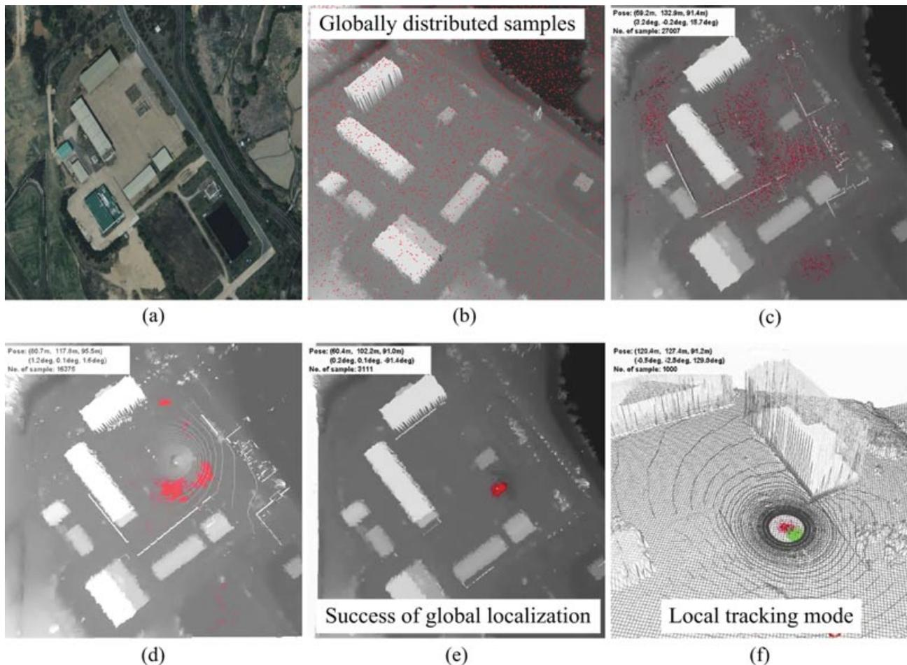
**Figure 19.** Experimental results from global localization using a Velodyne: (a) experimental environment and (b)–(f) sample convergence during global localization.
