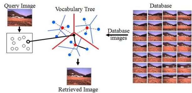
Fig. 3. The process of image retrieval and matching.
