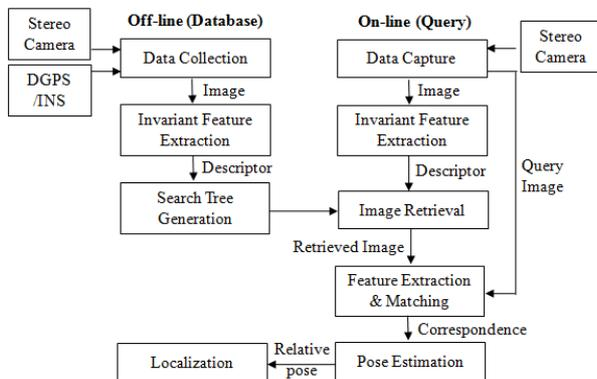
Fig. 2. Block diagram of visual localization algorithm.
