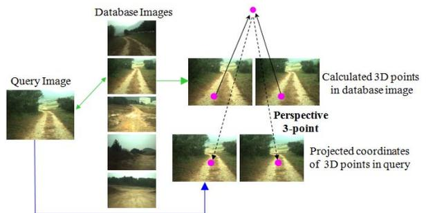
Fig. 4. The process of relative pose estimation.
