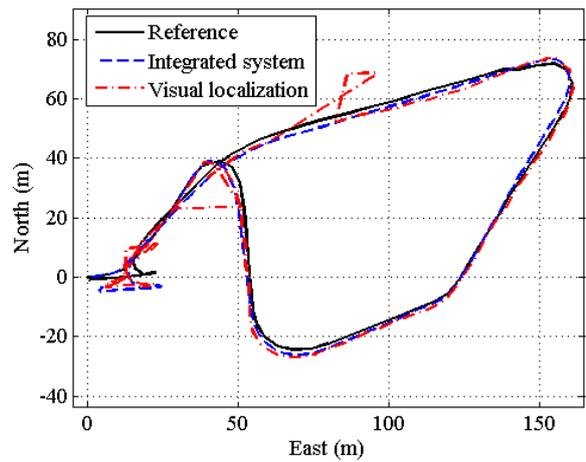
Fig. 17. Trajectory comparison: Path 2.
