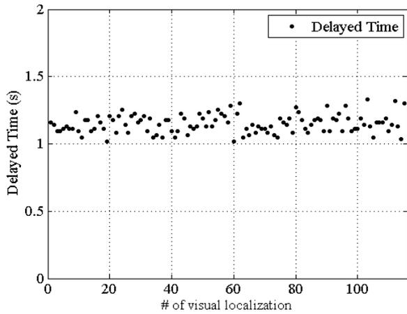
Fig. 14. Time delay of visual localization.
