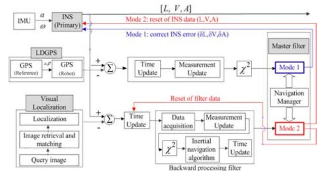
Fig. 10. Integrated localization system architecture.
