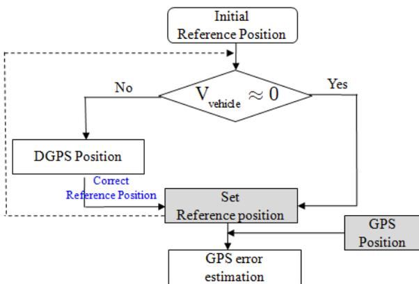
Fig. 6. LDGPS for the real-time reference position.
