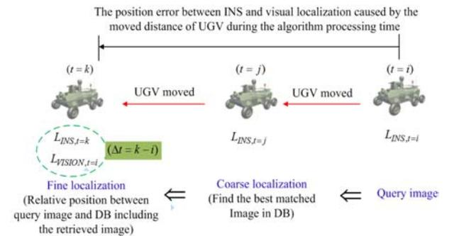
Fig. 7. Position error between two systems.
