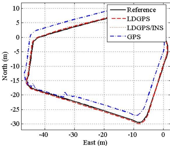
Fig. 11. Trajectory comparison: Mode 1.
