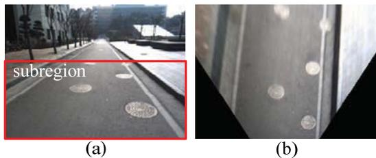
Fig. 2. Results of IPM: (a) original Image, and (b) top view of the original image transformed by IPM.
