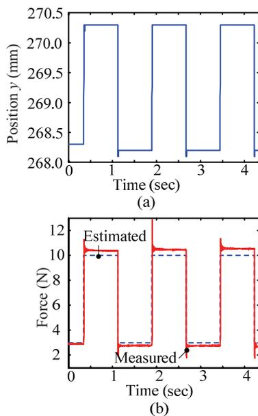
Fig. 8. Experimental results for stiffness estimation; (a) position of end-effector in the  $y$  direction, and (b) estimated and measured contact forces.
