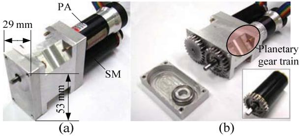
Fig. 2. Prototype of DAU; (a) DAU, and (b) internal view of DAU with planetary gear train.
