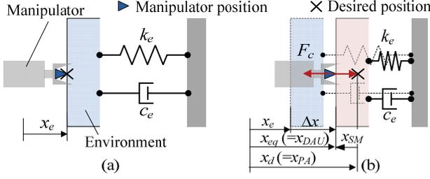
Fig. 4. Stiffness estimation using DAU.
