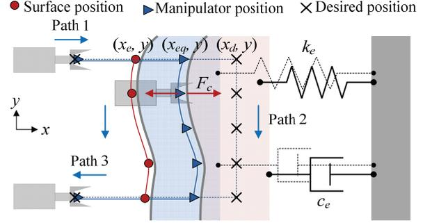
Fig. 5. Surface estimation by using DAU.
