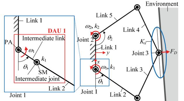
Fig. 6. Kinematic diagram of five-bar parallel manipulator with two DAUs
