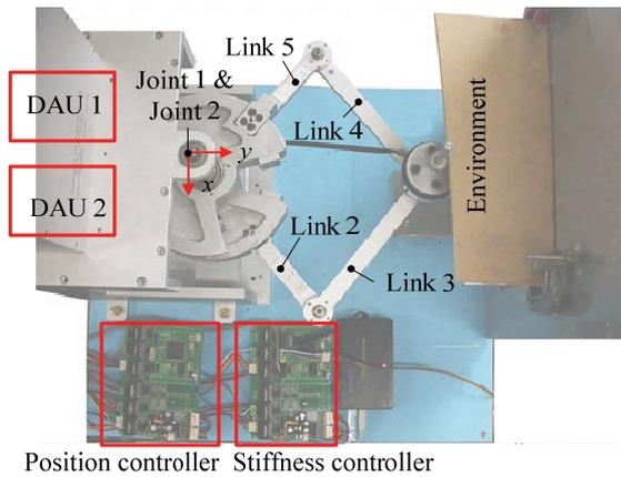
Fig. 7. Five-bar parallel manipulator with two DAUs
