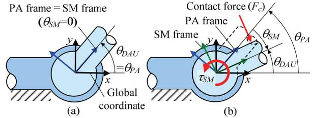
Fig. 3. Frames of PA and SM; (a) without contact force, and (b) with contact force.
