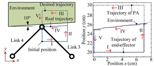
Fig. 9. Experimental results for surface estimation.
