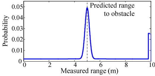
Fig. 4. Conventional sensor model for probability calculation based on difference between sensor data and predicted range data.
