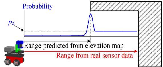
Fig. 7. Probability distribution by modified sensor model with elevation map.
