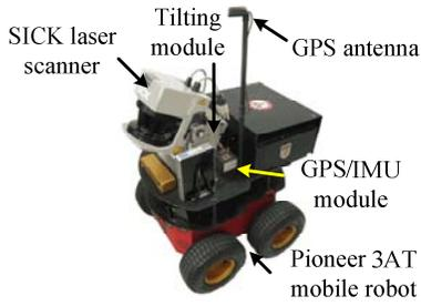
Fig. 8. Robot used for research.
