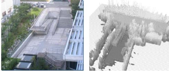
Fig. 9. Environment and reference elevation map.
