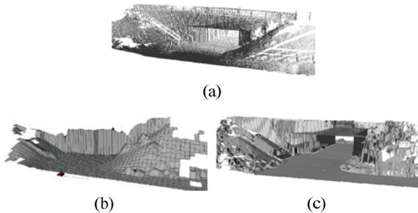
Fig. 1. Difference of map representation; (a) point clouds, (b) elevation map, and (c) multi-level surface map. (All figures are quoted in [4].)
