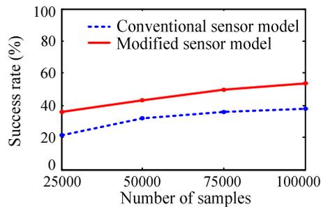
Fig. 11. Success rates of global localization by conventional and modified sensor models, respectively.
