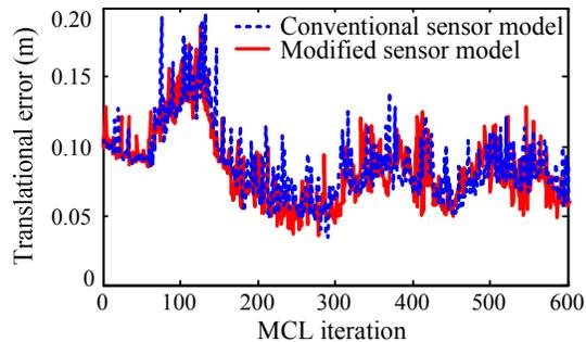
Fig. 12. Localization errors during local tracking with 1,000 samples.
