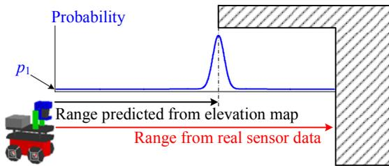
Fig. 5. Probability distribution by conventional sensor model with elevation map.
