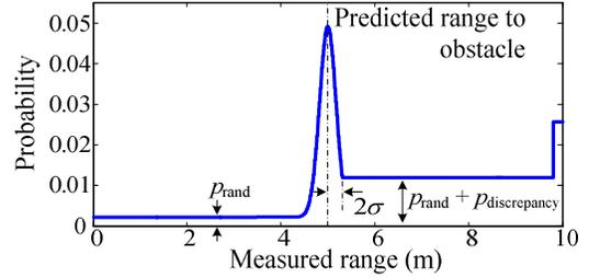
Fig. 6. Modified sensor model for probability calculation based on difference between sensor data and predicted range data.
