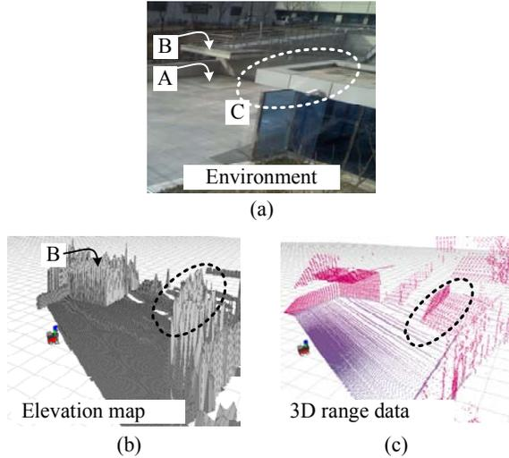
Fig. 2. Examples of discrepancy between elevation map and real range sensor data; (a) environment, (b) elevation map, and (c) real range sensor data.
