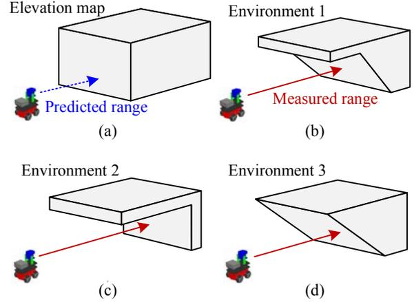
Fig. 3. Examples of environments to be modeled as an identical elevation map.
