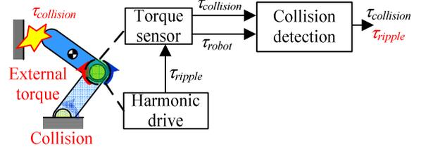
Fig. 1. The problem of torque ripple.
