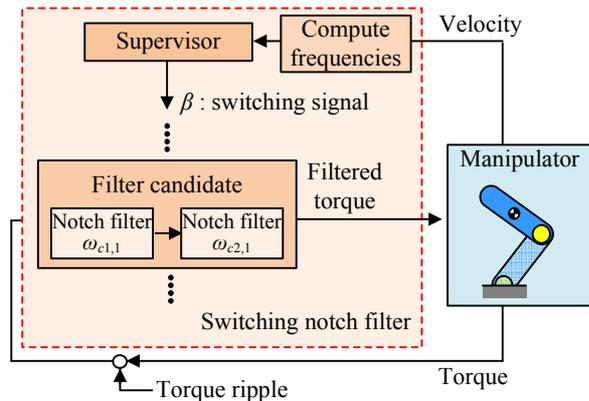
Fig. 2. Block diagram of the switching notch filter.
