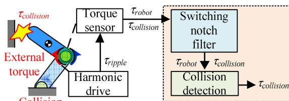
Fig. 3. The overall system with the switching notch filter.
