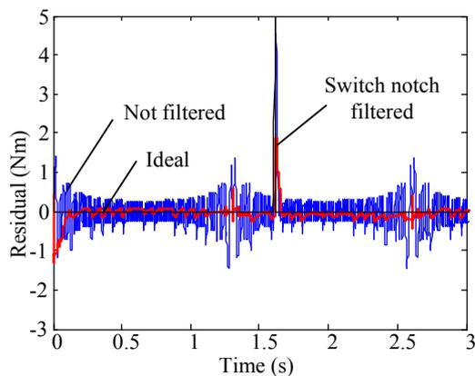
Fig. 6. The computed residuals with and without the switching notch filter.
