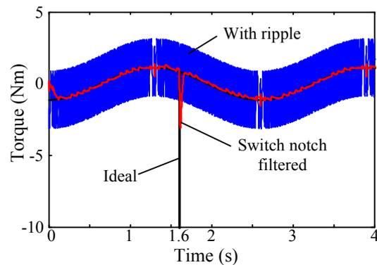
Fig. 5. Comparison between original, rippled, and filtered torques.
