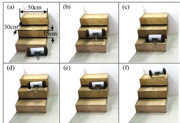
Figure 11 Experiments on stair climbing.
