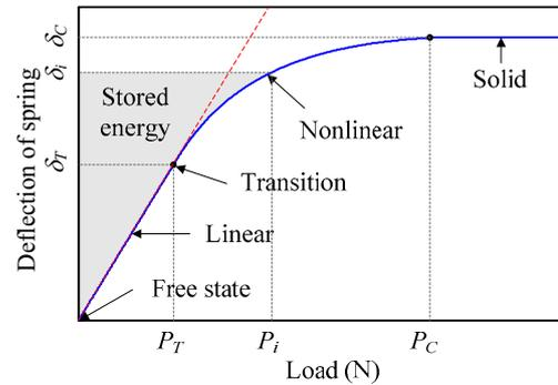
Figure 4 Graph of load-deformation relation.
