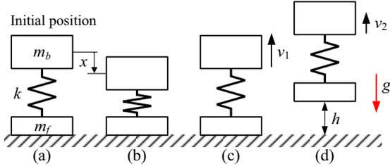
Figure 1 Jumping model; (a) initial state, (b) compressing, (c) releasing and (d) jumping.
