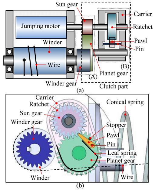
Figure 7 Jumping module; (a) top view, and (b) side view.
