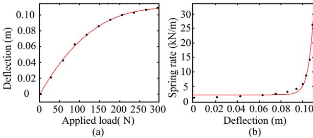
Figure 6 Experimental results; (a) load-deflection curve, and (b) deflection-spring rate curve.
