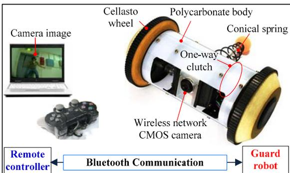
Figure 9 System of guard robot.
