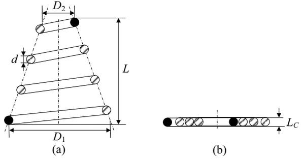
Figure 3 Conical spring: (a) initial state, and (b) fully compressed.
