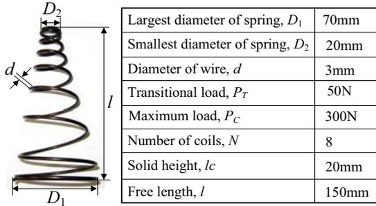
Figure 5 Manufactured conical spring and its specifications.
