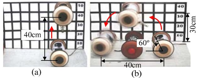
Figure 10 Jumping experiments; (a) vertical jumping and (b) jumping with jumping angle of 60°.
