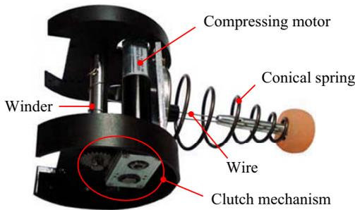
Figure 2 Jumping module composed of clutch mechanism and conical spring.
