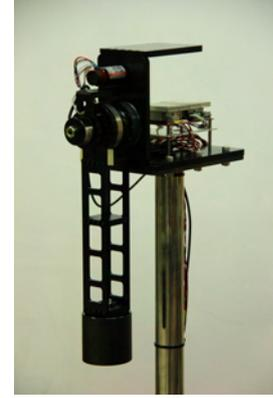
Fig. 4: One DOF flexible joint robot arm.
