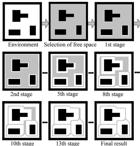
Fig. 2 Construction of a thinning-based topological map for given environment (Simulations).
