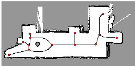
Fig. 11 Another example of grid and topological maps created by means of TTE in large-scale environment
