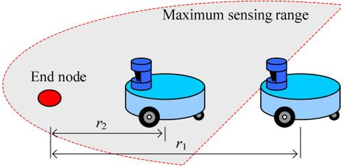
Fig. 6 A robot can scan the environment around the node at different distances.
