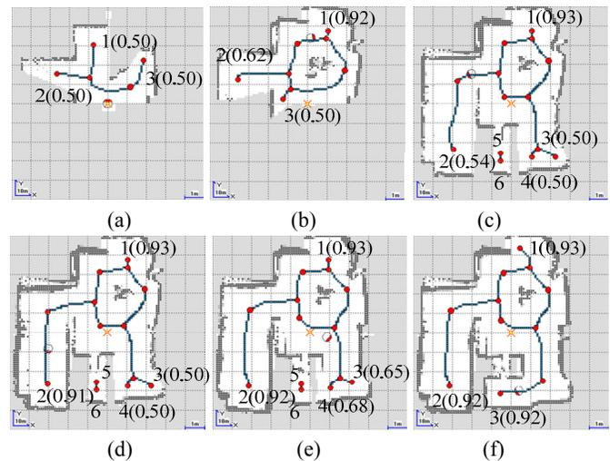
Fig. 9 Changes in end nodes and their probabilities during exploration.
