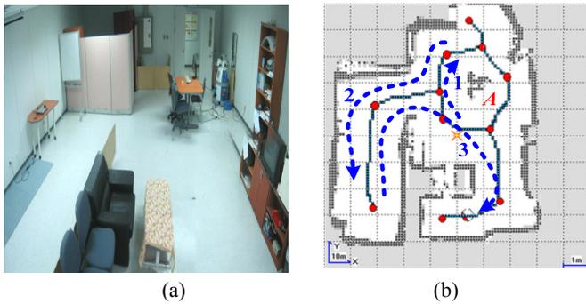
Fig. 10 (a) Experimental environment, and (b) grid and topological maps created using the TTE algorithm and robot paths during exploration.
