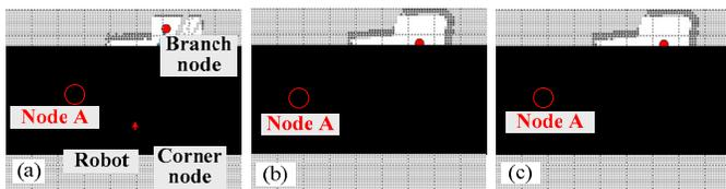
Fig. 4 Change in end node position during exploration of dead end of hallway.
