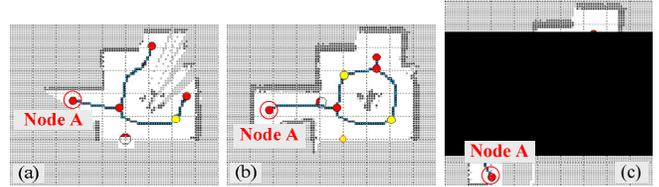
Fig. 5 Change in end node position during exploration of connecting area of two hallways.
