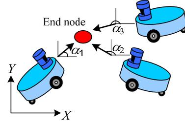
Fig. 7 A robot can scan the environment around the node from different angles.
