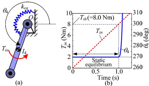
Fig. 5 Dynamic analysis of the nonlinear spring system; (a) free-body diagram, and (b) input torque and angular displacement of input link with time.
