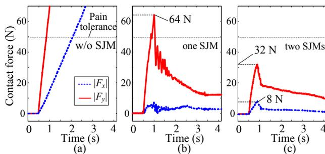
Fig. 14 Experimental results on static collision; (a) without SJM, (b) with one SJM-II, and (c) with two SJM-IIs.
