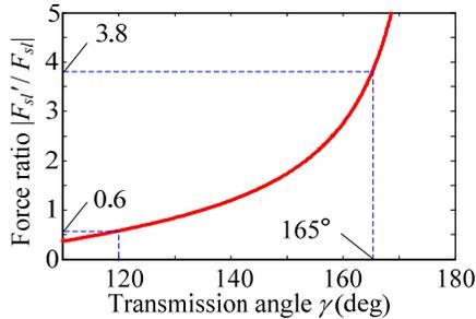
Fig. 2 Force ratio as a function of transmission angle.
