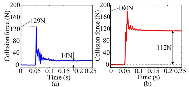
Fig. 12 Experimental results on dynamic collision; (a) with SJM-II, and (b) without SJM-II.
