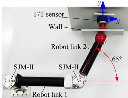
Fig. 13 Experimental conditions for collision safety of robot arm in 2-D space.
