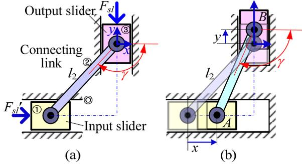
Fig. 1 (a) Double-slider mechanism, and (b) general configuration.
