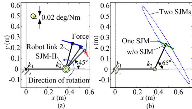
Fig. 8 Compliance ellipsoid of a robot arm equipped with SJM-II: (a) change of compliance according to external force, and (b) compliance when angle of joint 2 is  $65^\circ$ .
