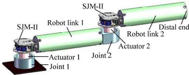
Fig. 7 2-DOF robot arm equipped with SJM.
