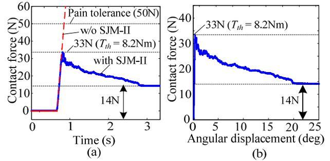
Fig. 11 Experimental results for static collision for robot arm: (a) collision force versus time with and without SJM-II, and (b) collision force versus angular displacement of SJM-II.
