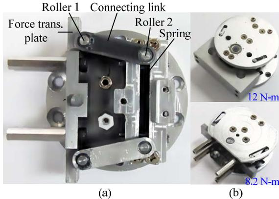
Fig. 9 Prototype of SJM-II: (a) internal view, and (b) two types of SJM-IIs.
