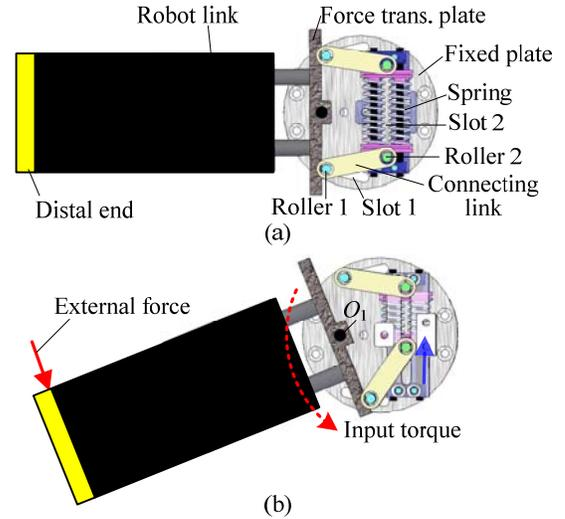
Fig. 6 Operation of SJM-II; (a) before collision, and (b) after collision.
