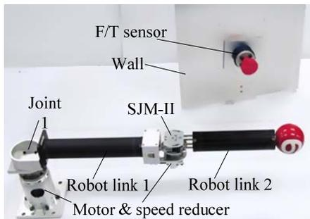
Fig. 10 Experimental setup for robot arm with SJM-II.
