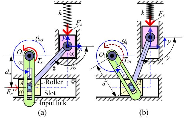
Fig. 3 Nonlinear spring system composed by a double-slider mechanism with a spring: (a) zero configuration, and (b) general configuration.
