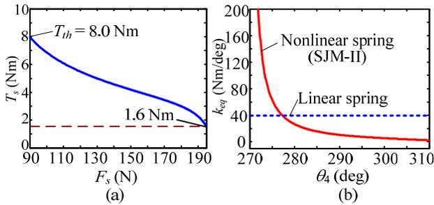
Fig. 4 (a) Spring torque versus spring force, and (b) equivalent stiffness of nonlinear spring system as a function of angle of input link.
