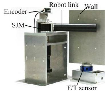
Fig. 11 Experimental setup for robot arm with SJM.
