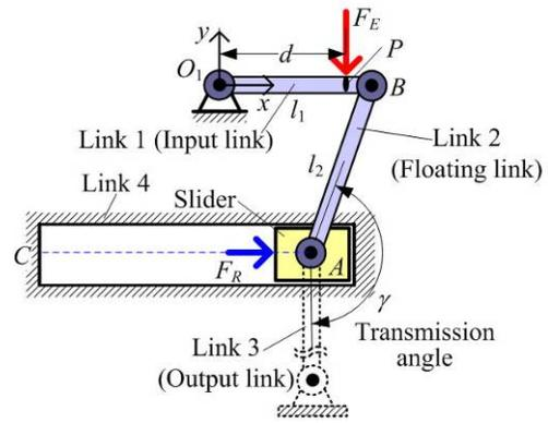
Fig. 2 Slider-crank mechanism.
