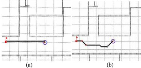
Fig. 9. Path passing through the junction ((a) conventional path (b) proposed path)
