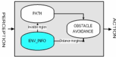
Fig. 8. The structure of safe navigation
