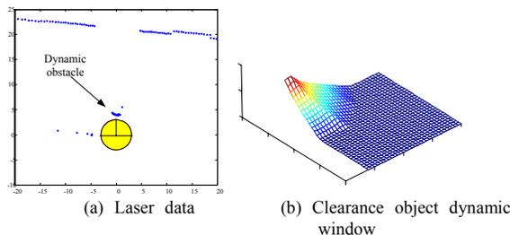
Fig. 13. Appearance of dynamic obstacle and the computed area of collision/collision-free velocities in dynamic window (left wheel velocity: 0.24m/s, right wheel velocity 0.34m/s)
