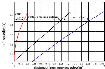
Fig. 5.  $d_{col}$  versus maximum safe speed of a robot
