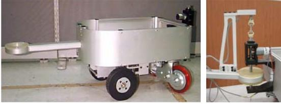
Figure 7. Passive off-hooked trailer (left) and potentiometer (right)
