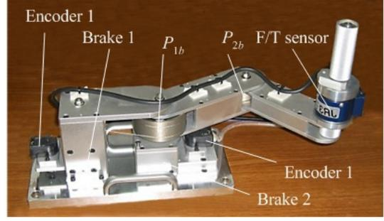
Fig. 8. Coupled tendon-drive mechanism.
