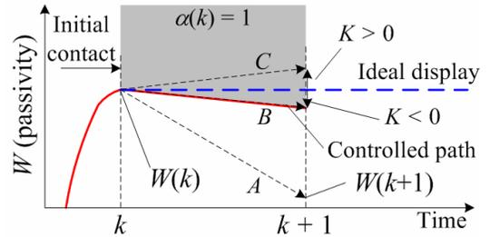
Fig. 7. Passivity plots as a function of time, showing the concept of passivity-based control.
