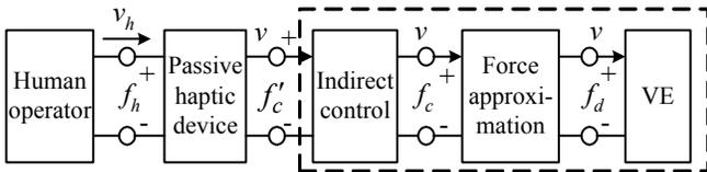
Fig. 6. Passive haptic interface system with delayed virtual environment.
