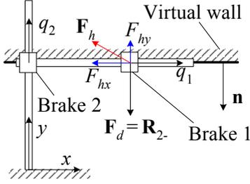
Fig. 3. X-Y table mechanism.
