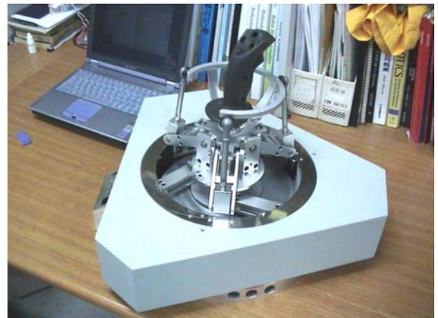
Fig 1. Overview of the haptic master
