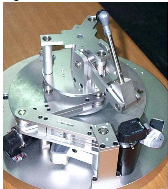
Fig 6. Tendon driven mechanism for power transmitting.
