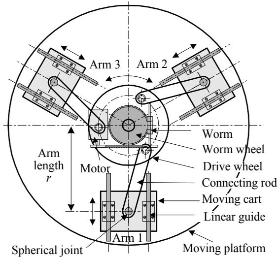
Fig. 2. Structure of variable arm mechanism.
