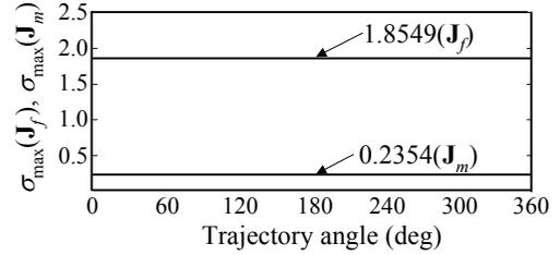
Fig. 12 Force-moment transmission gains for minimum arm length.
