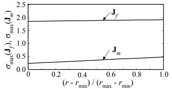
Fig. 13 Changes in force-moment transmission gains for continuously varying arm length.
