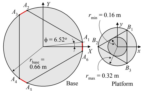
Fig. 4 Physical dimensions of fixed base and platform.
