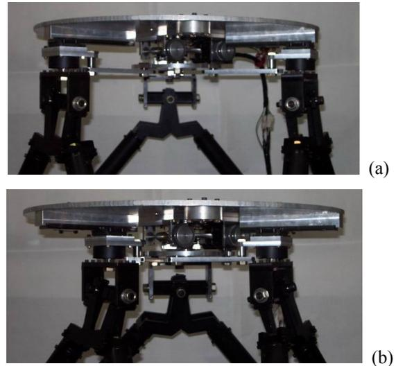
Fig. 3 Photos of variable arm type parallel manipulator: (a) maximum arm length, and (b) minimum arm length.
