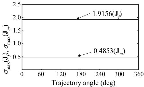
Fig. 11 Force-moment transmission gains for maximum arm length.
