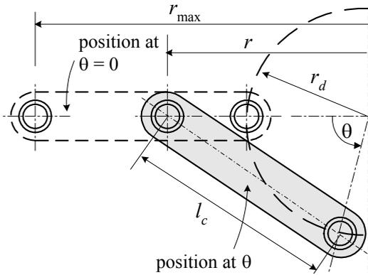
Fig. 5 Geometry of variable arm.
