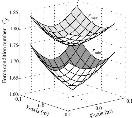
Fig. 14 Force condition number  $C_f$  at the maximum and minimum arm lengths on the XY plane.
