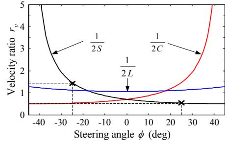
Fig. 7 Velocity ratio as a function of steering angle.
