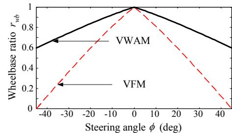
Fig. 4 Comparison of wheelbase ratios for variable wheel arrangement mechanism (VWAM) and variable footprint mechanism (VFM).
