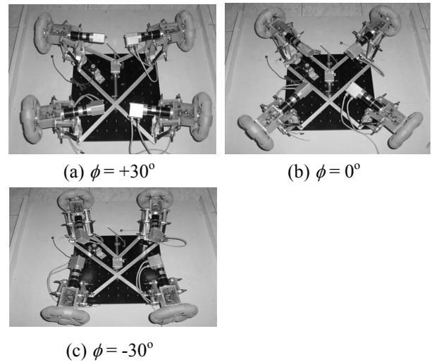
Fig. 3 Various wheel arrangements using variable wheel arrangement mechanism.
