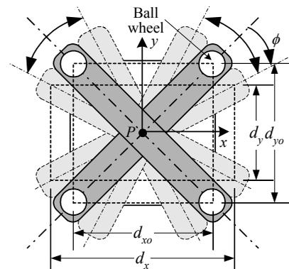
Fig. 1 Variable footprint mechanism for CVT [9].
