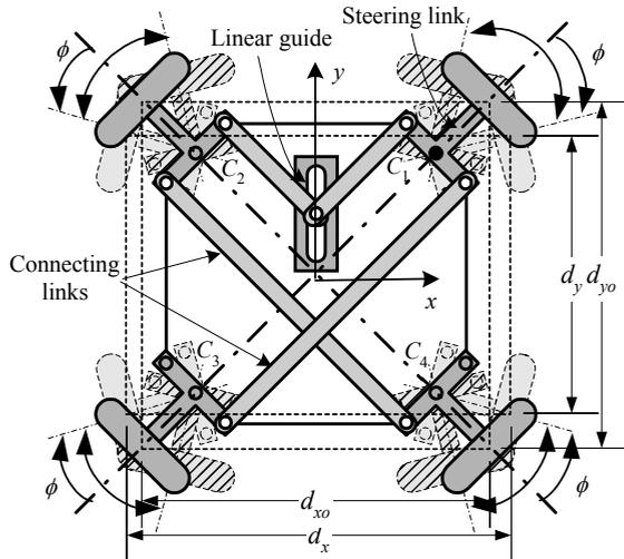
Fig. 2 Variable wheel arrangement mechanism for CVT.
