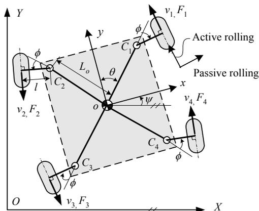
Fig. 5 Coordinate systems for omnidirectional mobile robot under consideration
