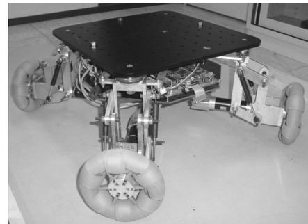
Fig. 10 Omnidirectional mobile robot
