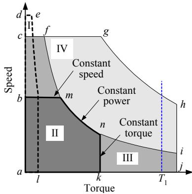
Fig. 9 Operating regions of motor (I: motor, II: motor + speed reducer, III: motor + speed reducer + CVT, IV: large motor + speed reducer)
