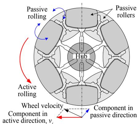
Fig. 6 Appearance of continuous alternate wheel and active and passive rolling.
