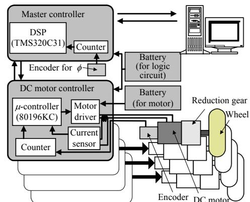
Fig. 11 Control systems for mobile robot
