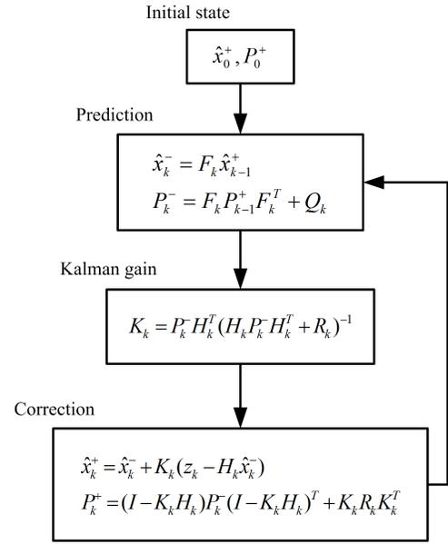
Fig. 4. Block diagram of the process of the Kalman filter
