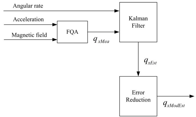
Fig. 8. the block diagram of the design for estimating the orientation
