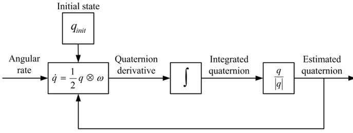
Fig. 3. Block diagram of the process for the orientation represented in quaternion
