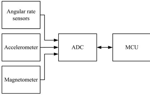
Fig. 1. Block diagram of the sensor module
