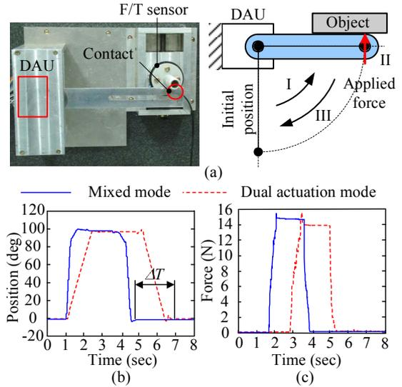
Fig. 11 Step responses for three modes: (a) position of link and (b) measured force at object
