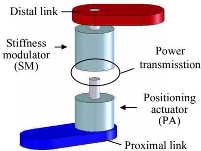
Fig. 2 Two actuators connected in series
