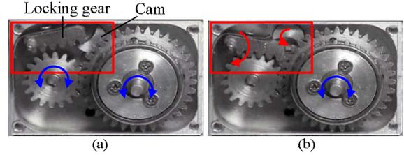
Fig. 8 Clutch mechanism; (a) released, and (b) locked.
