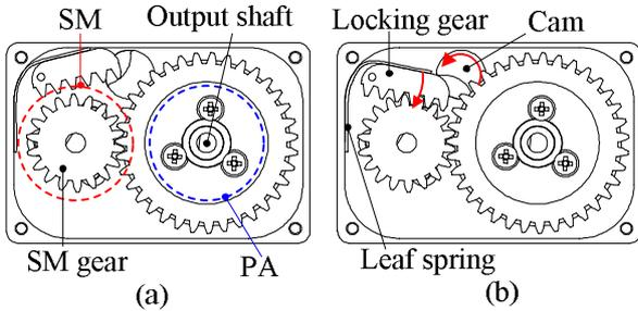
Fig. 6 Clutch mechanism for high torque mode; (a) before clutching, and (b) after clutching.
