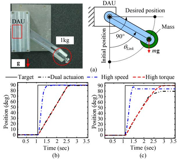
Fig. 9 Step responses for three modes: (a) experimental setup, (b) with no-load, and (c) with load.
