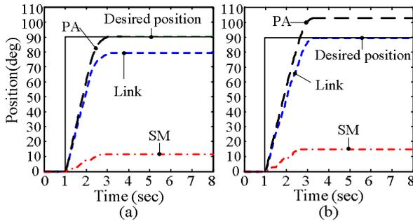
Fig. 10 Experimental results for compensation of PA; (a) without compensation, and (b) with compensation.
