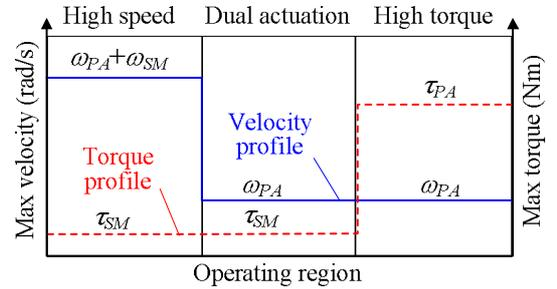
Fig. 4 Velocity and torque profiles for each mode
