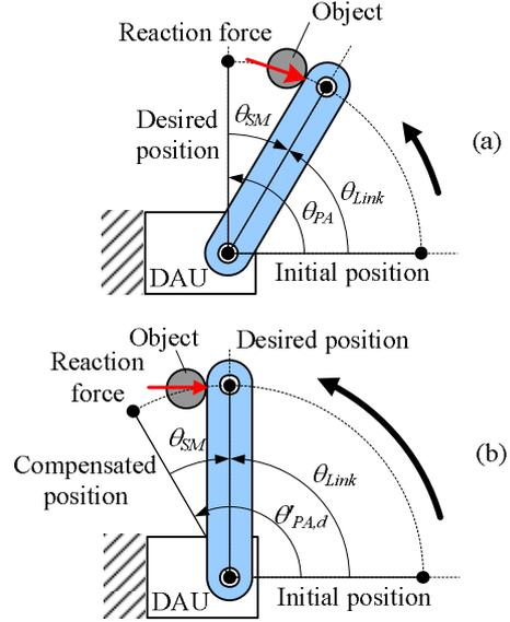
Fig. 5 Compensation for PA position in dual actuation mode; (a) before compensation, and (b) after compensation.
