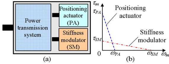
Fig. 1 DAU; (a) conceptual diagram of DAU, and (b)  $T_m$ - $\omega_m$  curve for each motor
