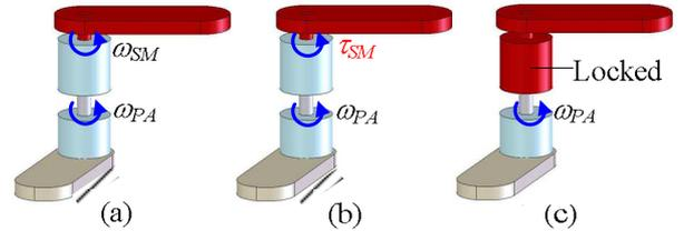
Fig. 3 Schematics of three modes of DAU; (a) high speed mode, (b) dual actuation mode, and (c) high torque mode.
