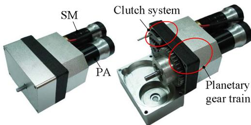
Fig. 7 Prototype of DAU with cam-based clutch system
