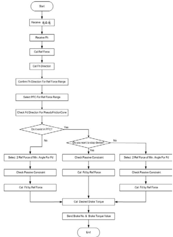
Fig. 8 Brake Torque Generation Flow chart
