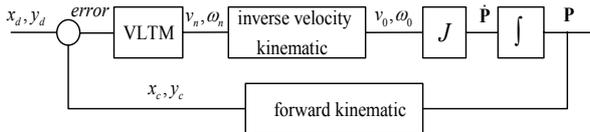
Fig. 4 Architecture of proposed tracking control method
