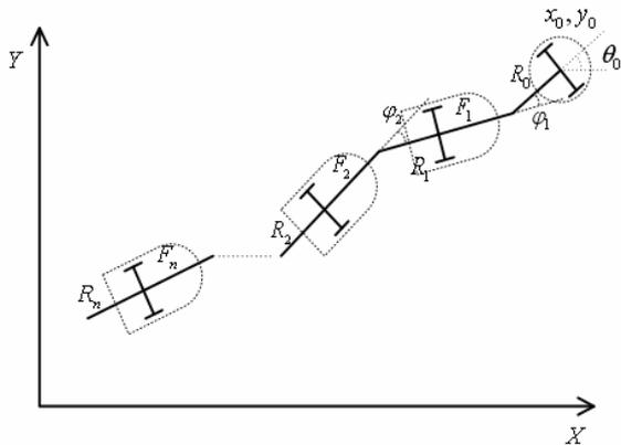
Fig. 2 Kinematic model
