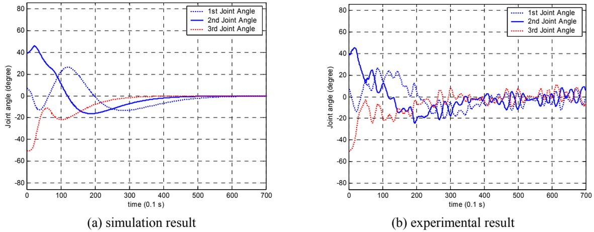
Fig. 9 Relative angles between trailers
