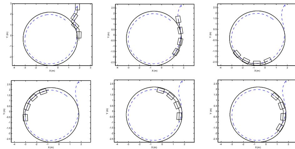
Fig. 7 Experimental result : a Circle path ( radius = 2.5 m )
