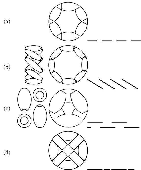
Fig. 1 Various wheel types using passive rollers and their traces; (a) classic, (b) Mecanum, (c) double, and (d) alternate.
