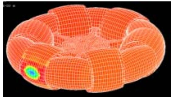
Fig. 10 Stress distribution of outer roller of wheel subject to a vertical load of 50kg
