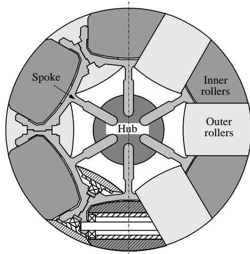
Fig. 8 Schematic diagram of proposed continuous alternate wheel
