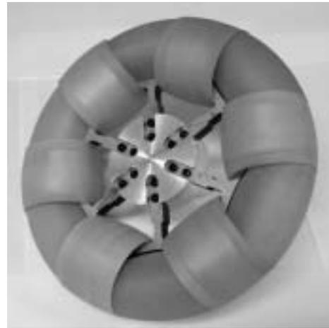
Fig. 9 Photo of constructed continuous alternate wheel
