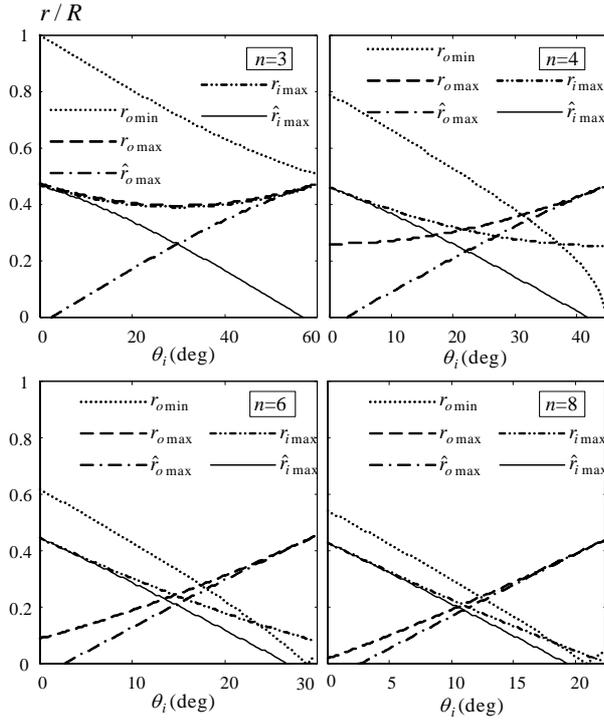
Fig. 5 Roller radii as a function of  $\theta_i$  for various values of  $n$
