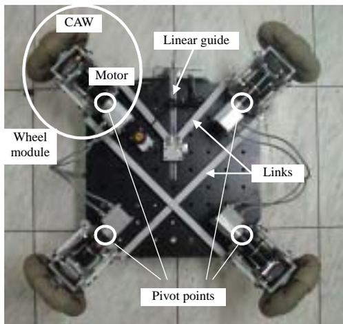
Fig. 11 Bottom view of prototype vehicle with CAWs
