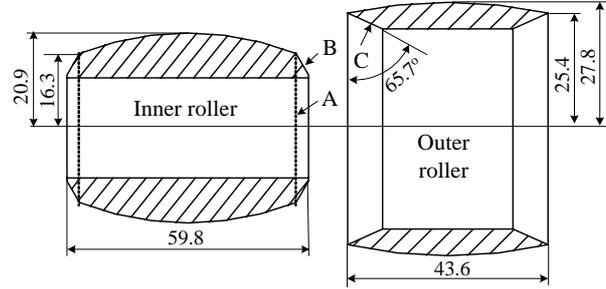
Fig. 6 Final shapes of inner and outer rollers
