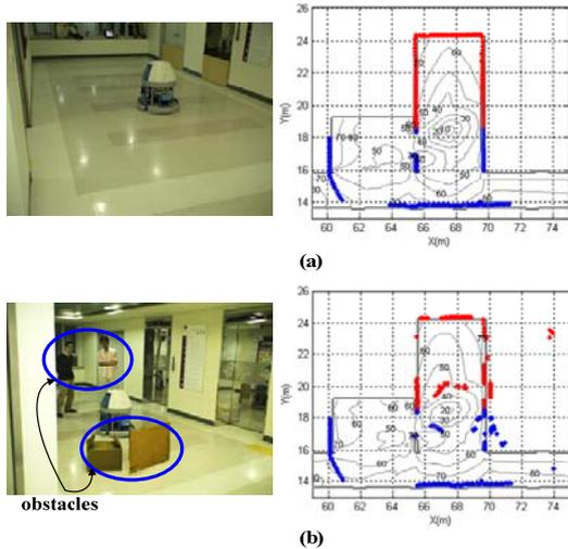
Fig. 7. *Matching error* contour by corruption of sensor data by obstacles. (a) *Corruption ratio* 0% (b) *Corruption ratio* 30%
