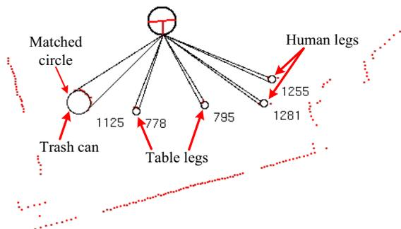
Fig. 4 Detection of arcs based on Hough transform.
