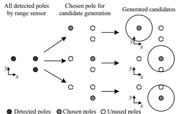
Fig. 6 Example of candidate generation of model  $A$ .
