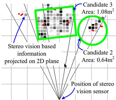
Fig. 9 Evaluation using candidate size and stereo vision based information.
