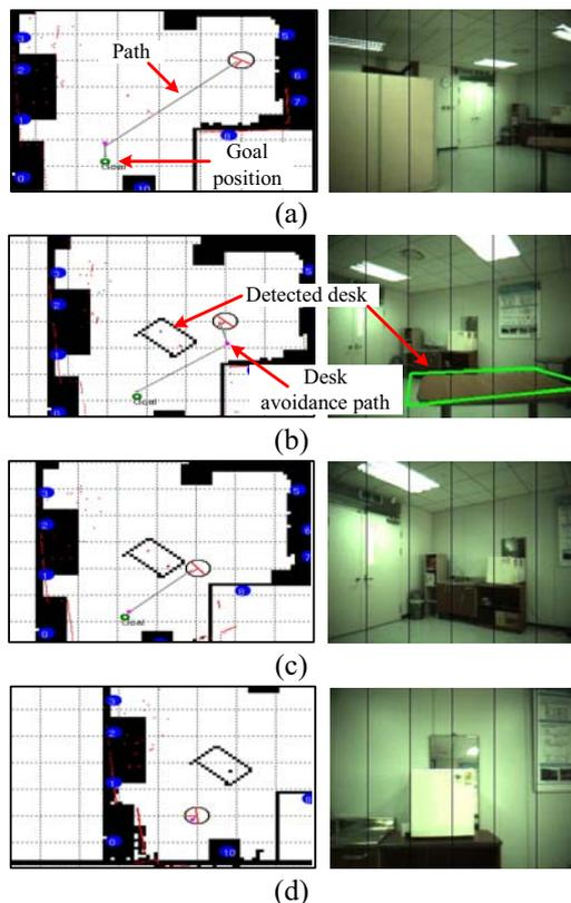
Fig. 12 Experiments on table detection and avoidance in real environment. Left figures show map and path, and right figures show images obtained from vision sensor.
