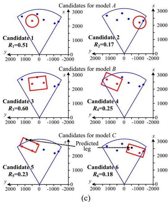
Fig. 8 Examples of some candidates in real environment using model A, B and C; (a) visual image and some stereo vision based information, (b) positions of 6 detected poles, and (c) some of candidates generated using model information and positions of poles.
