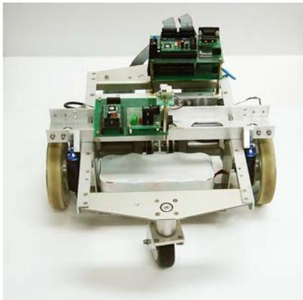
Fig. 6 Mobile Robot with IRID Receiver
