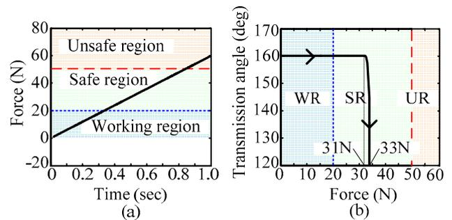
Fig. 8 Simulation results for static collision for initial transmission angle of  $160^\circ$ ; (a) external force versus time, and (b) transmission angle versus external force.
