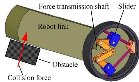
Fig. 7 Modeling of safety mechanism.
