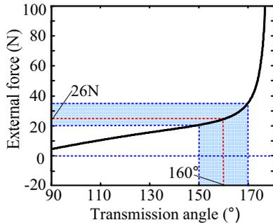
Fig. 4 External force as a function of transmission angle.
