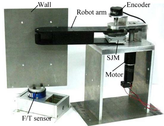
Fig. 10 Experimental setup for robot arm with SJM.
