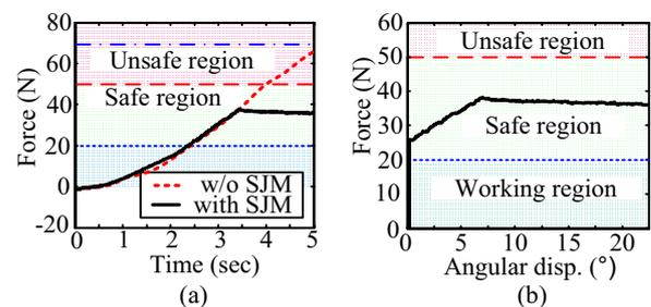
Fig. 11 Experimental results for static collision for robot arm; (a) collision force versus time without and with SJM, and (b) collision force versus angular displacement of SJM.
