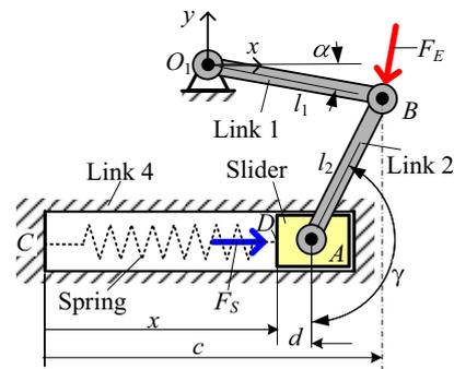
Fig. 3 Slider-crank mechanism combined with spring.
