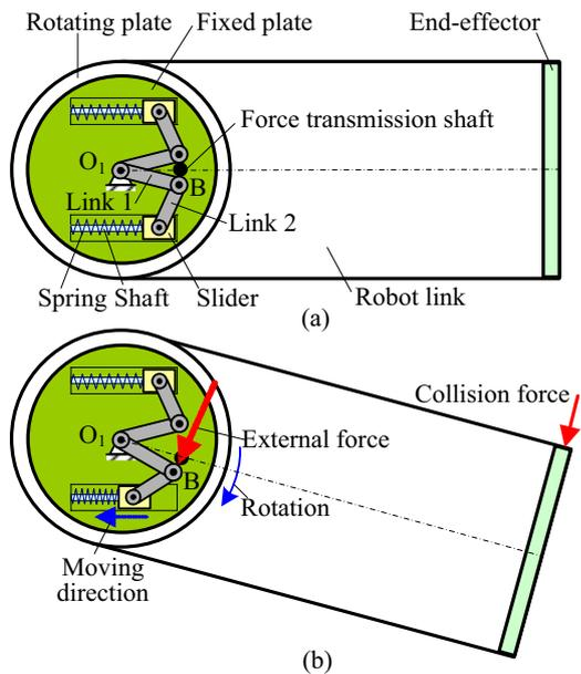
Fig. 6 Operation of SJM; (a) before collision, and (b) after collision.
