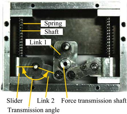
Fig. 9 Prototype of SJM.
