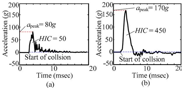
Fig. 12 Experimental results for dynamic collision of robot arm; acceleration versus time (a) with SJM, and (b) without SJM.
