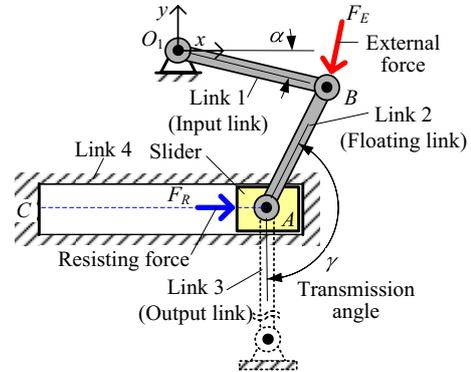
Fig. 2 Slider-crank mechanism.
