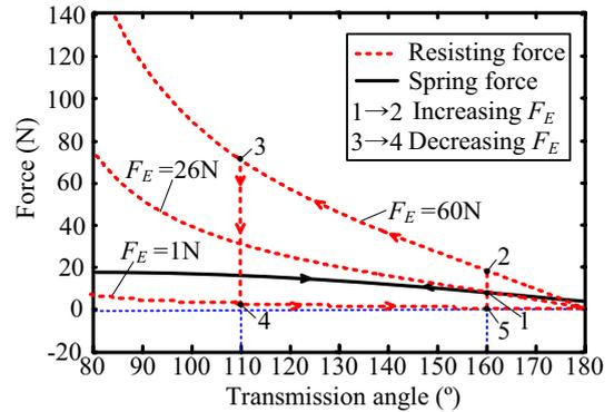
Fig. 5 Plots of resisting force and spring force versus transmission angle for high and low critical impact forces.
