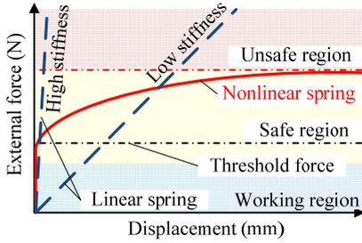
Fig. 1 Comparison between linear and nonlinear spring.
