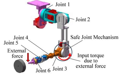
Fig. 5 6 DOF humanoid arm with safe joint mechanism.
