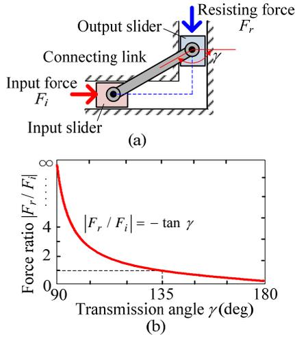
Fig. 2 Double slider mechanism: (a) simplified model, and (b) force ratio vs. transmission angle.
