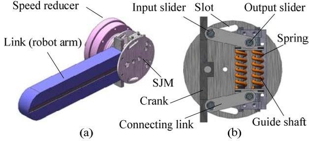
Fig. 8 Model of SJM-II; (a) installation of SJM-II at joint 3, and (b) structure of SJM-II.
