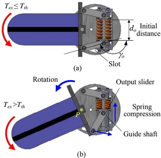
Fig. 9 Operation of SJM-II with external force; (a) before collision, and (b) after collision.
