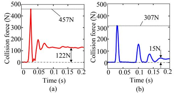
Fig. 13 Experimental results on dynamic collision; (a) without SJM-II, and (b) with SJM-II.
