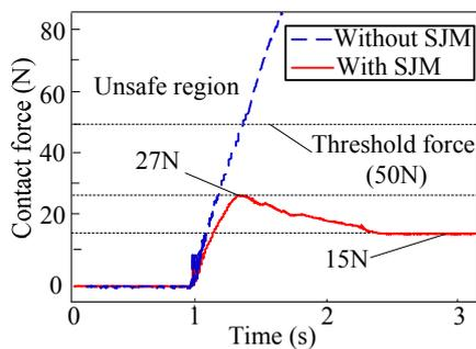
Fig. 12 Experimental result of static collision
