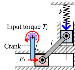
Fig. 7 Modified double slider mechanism with spring.
