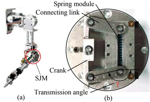
Fig. 10 Prototype of SJM-II; (a) humanoid arm with SJM-II, and (b) construction of SJM-II.
