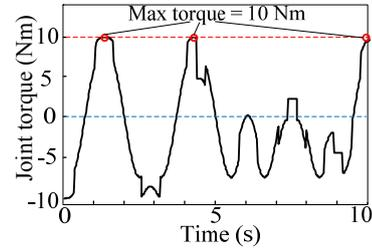
Fig. 6 Torque required for joint 3 in dynamic operation.
