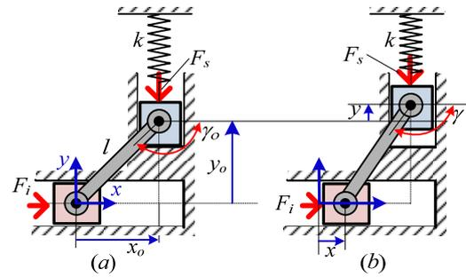
Fig. 3 Double slider mechanism with spring for realization of nonlinear stiffness: (a) zero configuration, and (b) general configuration.
