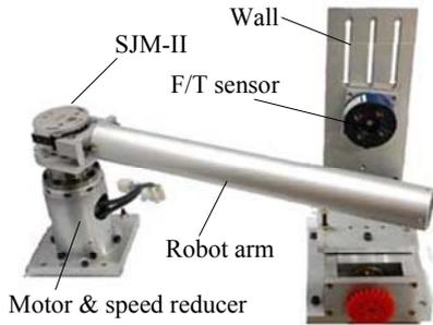
Fig. 11 Experimental setup for 1 DOF robot arm with SJM-II.
