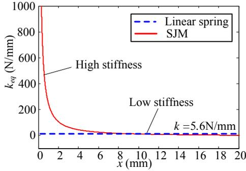
Fig. 4 Nonlinear stiffness of SJM as a function of displacement.
