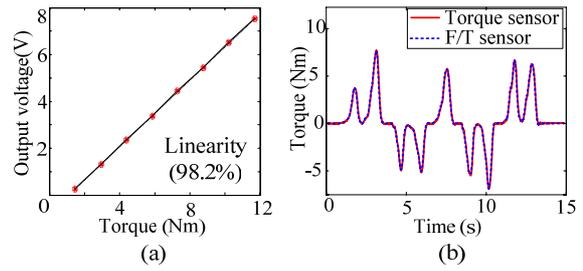
Fig. 11 Comparison between designed torque sensor and commercial F/T sensor: (a) linearity and torque coefficient, and (b) torque with random input.
