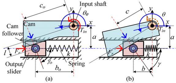
Fig. 2 Cam and Cam-follower mechanism for nonlinear stiffness: (a) zero configuration, and (b) general configuration.
