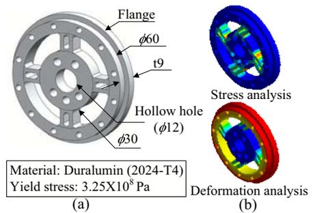
Fig. 4 Design of embedded joint torque sensor: (a) 3D modelling, and (b) stress and deformation analysis (FEM analysis).
