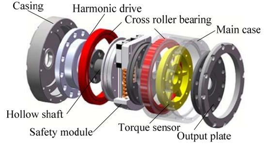
Fig. 7 Structure of proposed safe joint module.
