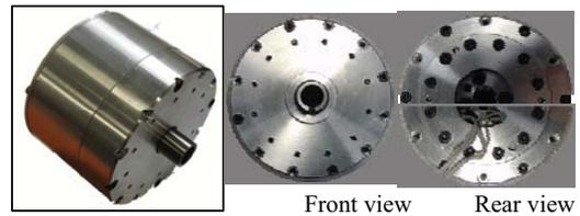
Fig. 9 Prototype of safe joint module.
