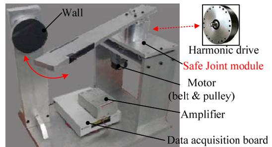
Fig. 12 Experimental setup for 1-DOF robot arm with and without safe joint module.
