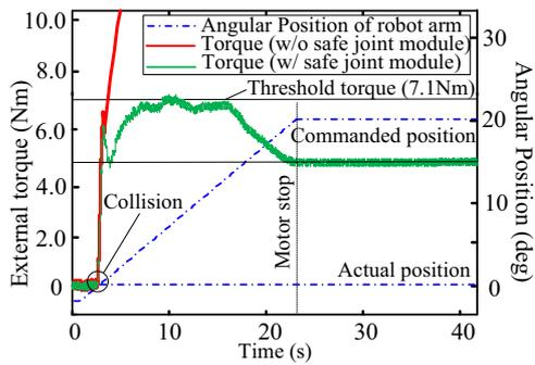
Fig. 13 Experimental results with static collision to verify nonlinear stiffness characteristic of proposed mechanism.
