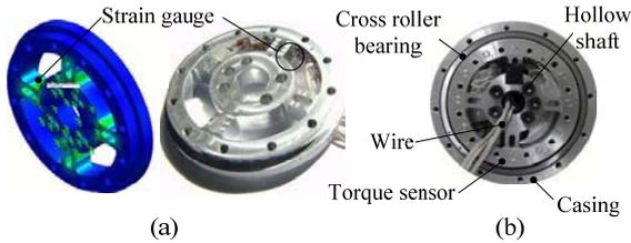
Fig. 6 Construction of embedded joint torque sensor: (a) Position for strain gauge and prototype, and (b) installation of torque sensor.
