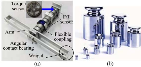
Fig. 10 Experimental setup for performance test of embedded torque sensor: (a) experimental setup, and (b) weight.
