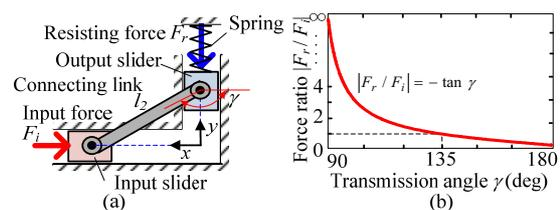
Fig. 1 Double-slider mechanism: (a) simplified model, and (b) force ratio vs. transmission angle.
