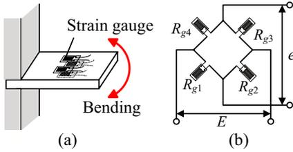
Fig. 5 Measurement of bending: (a) installation of strain gauges for torque measurement, and (b) full-bridge circuit.
