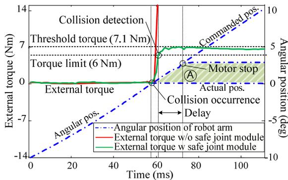
Fig. 14 Experimental results with dynamic collision with and without safe joint module.
