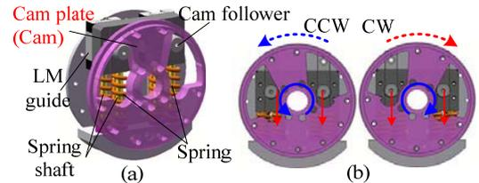
Fig. 8 Design of safety mechanism: (a) Structure of safety mechanism, and (b) operation after collision.
