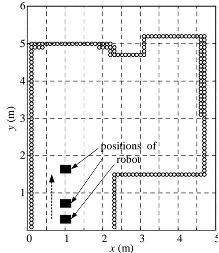
Fig. 7 Global grid map and sensing position.
