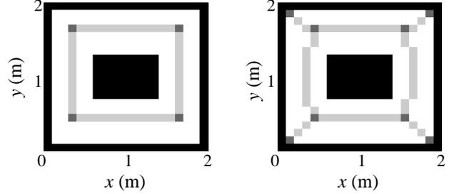
Fig. 4 Topological map using Voronoi diagram (left) and thinning method (right).
