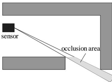
Fig. 6 Occlusion due to sensor limitation.
