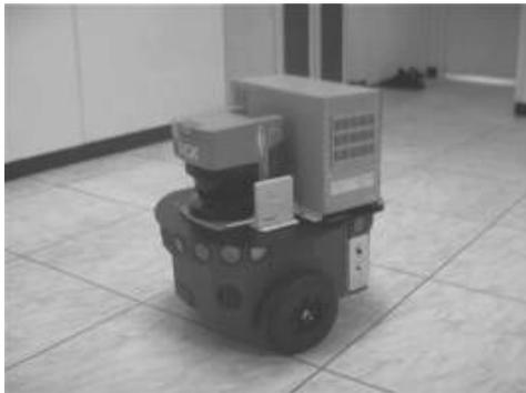
Fig. 9 Pioneer 2-DX mobile robot equipped with ultrasonic sensors and PC.
