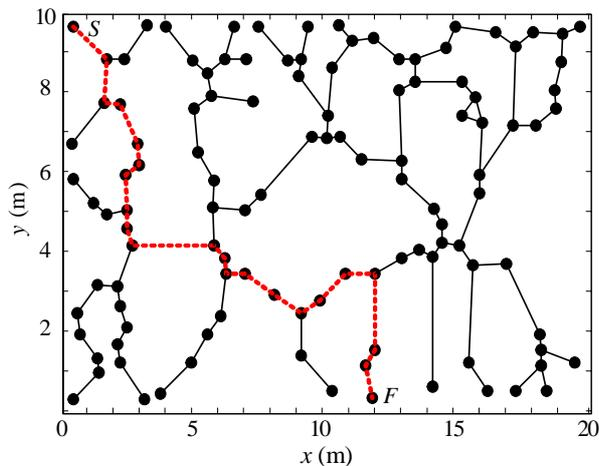
Fig. 14 Optimal path planning (from S to F).
