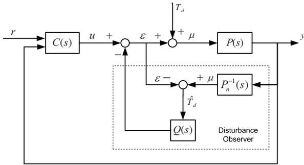
Fig. 4: Block diagram of proposed controller
