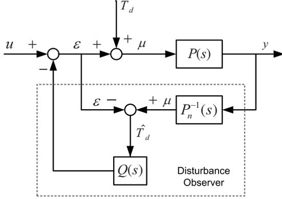
Fig. 2: Basic concept of disturbance observer
