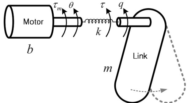
Fig. 1: 1 D.O.F. Flexible joint robot
