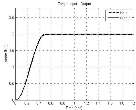
Fig. 6: Step response of PD + DOB controller: desired(dashed) and measured(solid)
