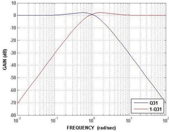
Fig. 3: Bode Plot of  $Q(s)$ : when  $f_c = 0.01s$ .
