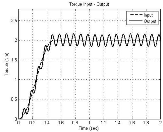
Fig. 5: Step response for PD controller: desired(dashed) and measured(solid)
