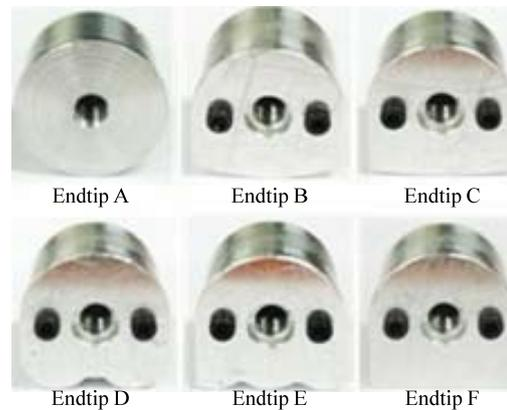
Fig. 6 Various types of endtip nuts.
