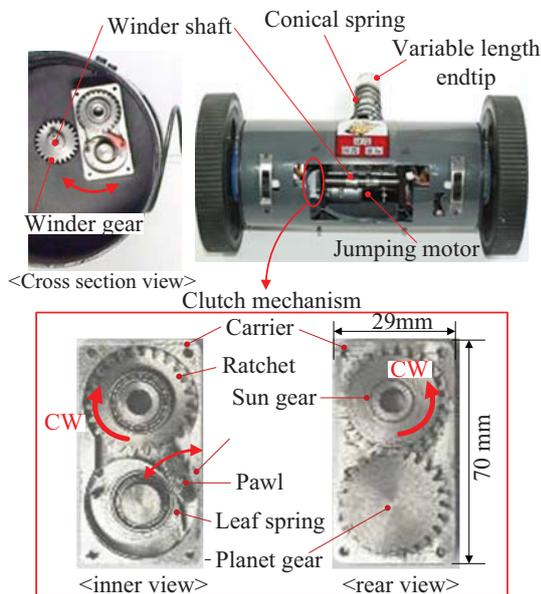
Fig. 2 Jumping mechanism.
