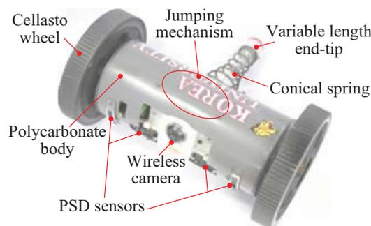
Fig. 1 Jumping robot based on conical spring.
