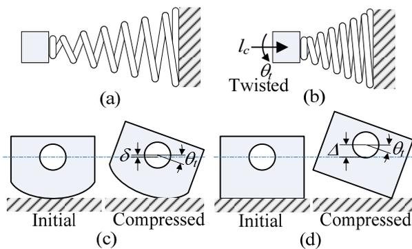
Fig. 8 Twisting of coil spring: (a) initial state of spring, (b) compressed state of spring, (c) circular endtip, and (d) rectangular endtip.
